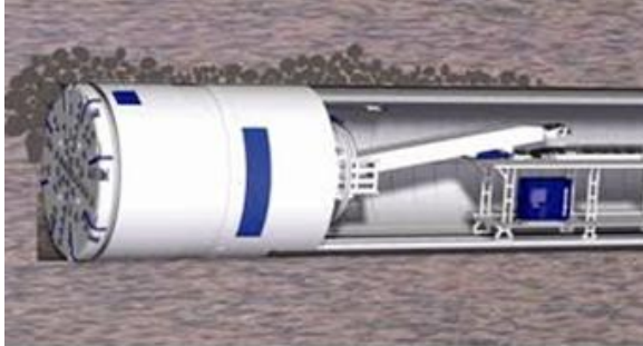
Shield Tunneling Method
