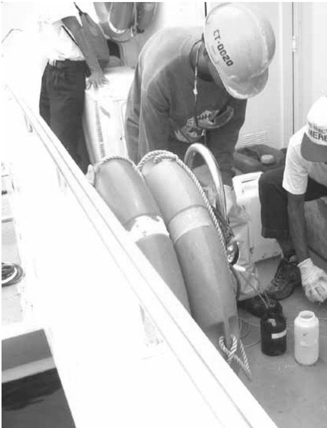
Preparation of sampling containers for the joint MIRANT Pagbilao and MMT quarterly marine water quality monitoring survey.
