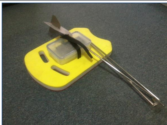
Plate 2.2.18. Drifter set-up used to track sub-surface current trajectory
