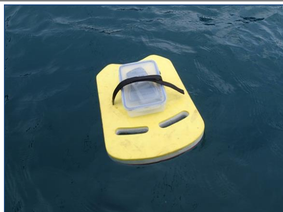
Plate 2.2.19. Actual use of drifter with the submerged stainless fins to track sub-surface current trajectory
