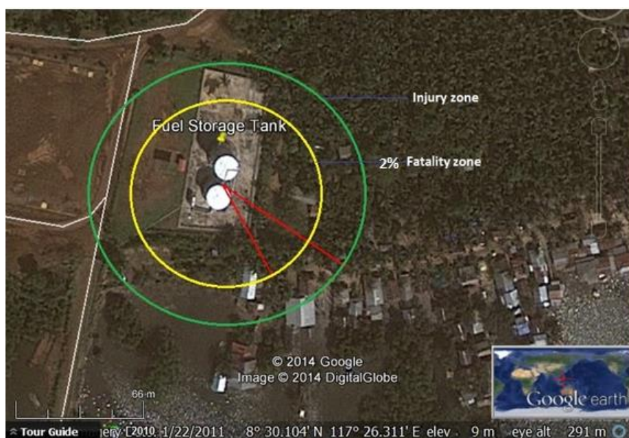
Figure 3.4.3. Potential injury and fatality zones resulting from bundled diesel pool fire
