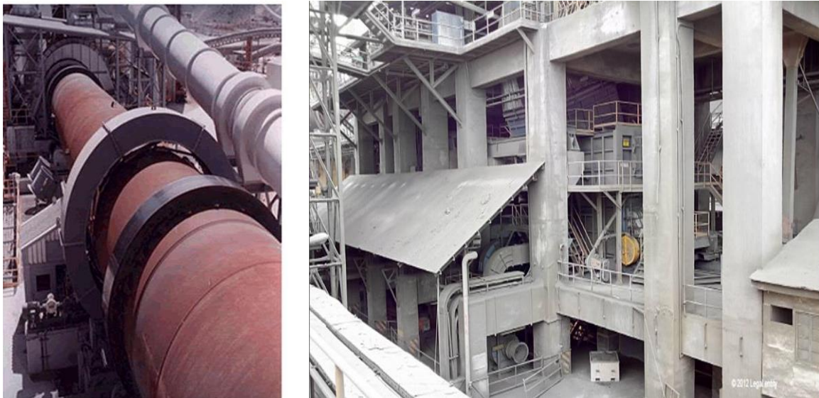
Plate 5: Kiln being used in clinker production ( left photo ); IKN Pendulum Clinker Coller ( right photo )
