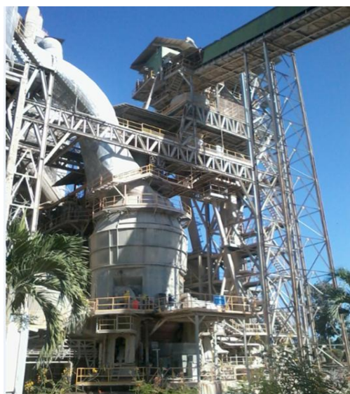
Plate 4: Fuller vertical roller mill being used for raw material grinding.
