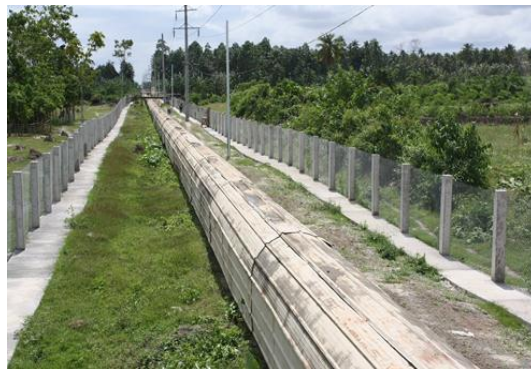
Plate 3: Crusher materials is conveyed to the plant through a 7 km belt conveyor at 500 tph
