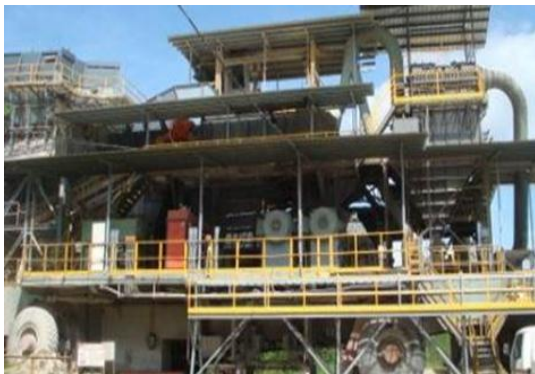
Plate 3: Crusher materials is conveyed to the plant through a 7 km belt conveyor at 500 tph
