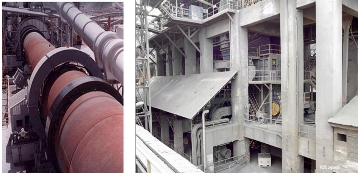
Plate 5: Kiln being used in clinker production ( left photo ); IKN Pendulum Clinker Coller ( right photo )
