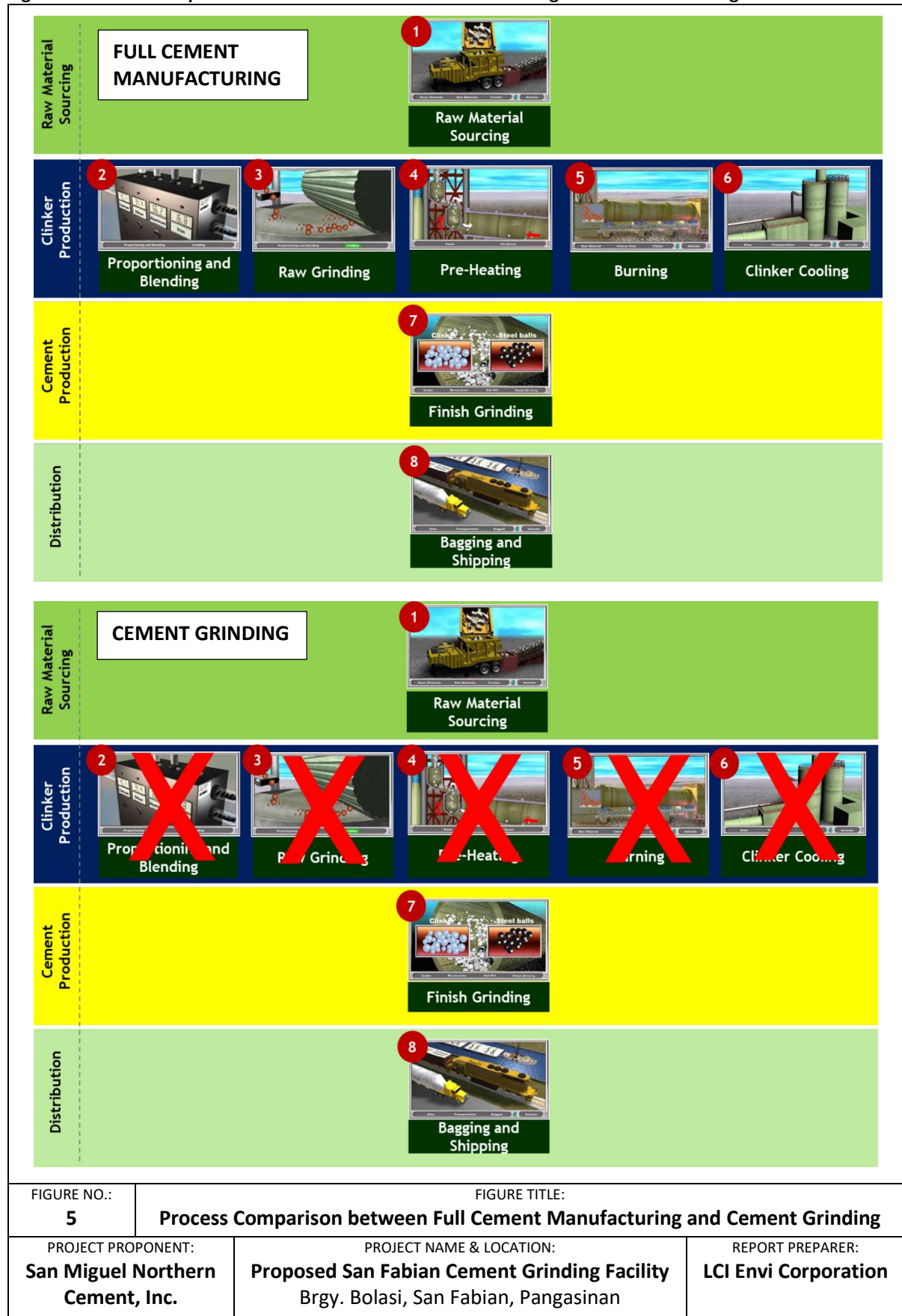
Figure 5: Process Comparison between Full Cement Manufacturing and Cement Grinding
