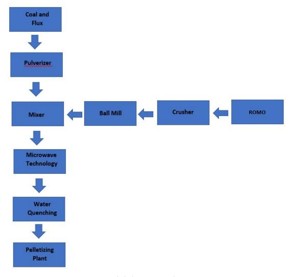
Figure 7 - Ferro-Nickel Plant Process Flow
