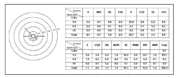
Figure 117 - Wind Rose Diagram and Frequency Table for Iba, Zambales from 1971-2000 (Annual)
