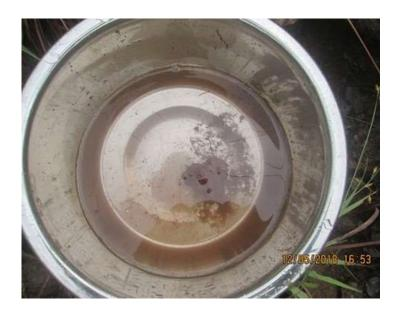
Figure 41 - Start of Slake Test P2 SS6
