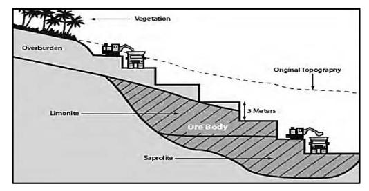
Figure 8 - Section of a Contour Mining Method
