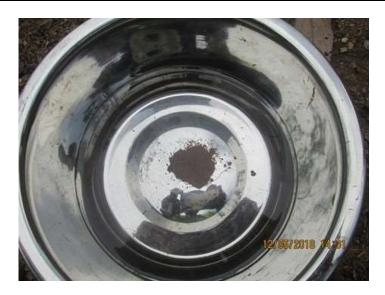
Figure 39 - Start of Slake Test P8 SS5
