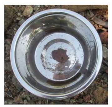
Figure 31 - Start of Slake Test, P7 SS1
