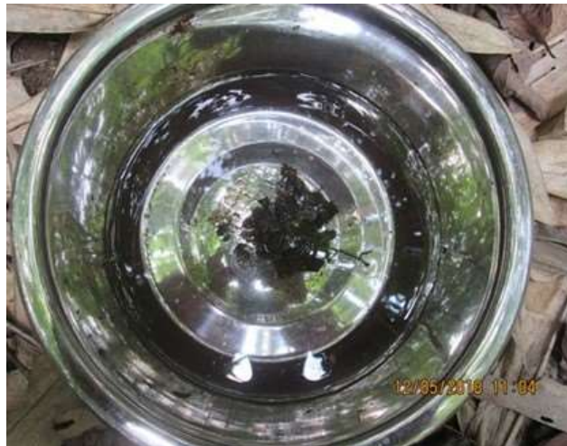
Figure 40 - End of Slake Test P2 SS3
