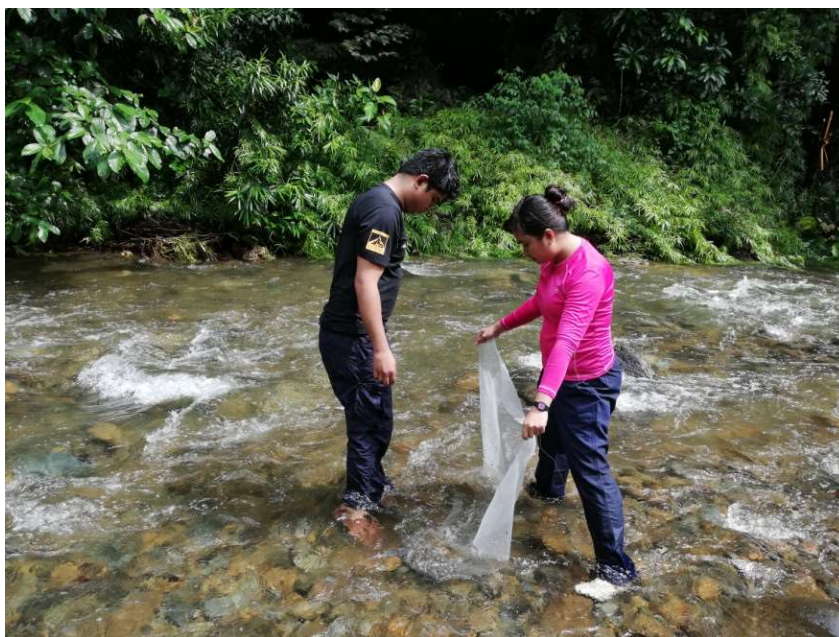
Plate 19 - Benthic macroinvertebrates collection using rectangular kick net
