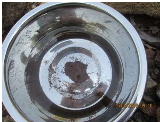
Figure 36 - End of Slake Test, P7 SS1
