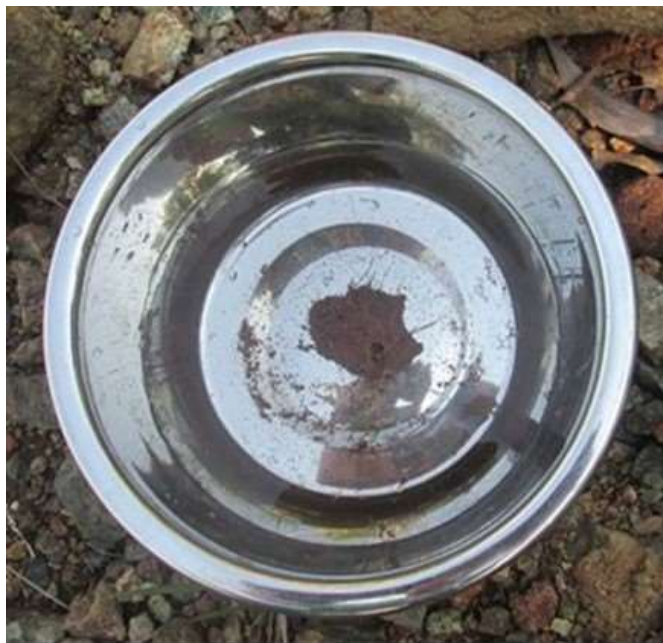
Figure 35 - Start of Slake Test, P7 SS1
