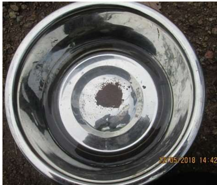
Figure 44 - End of Slake Test P8 SS5
