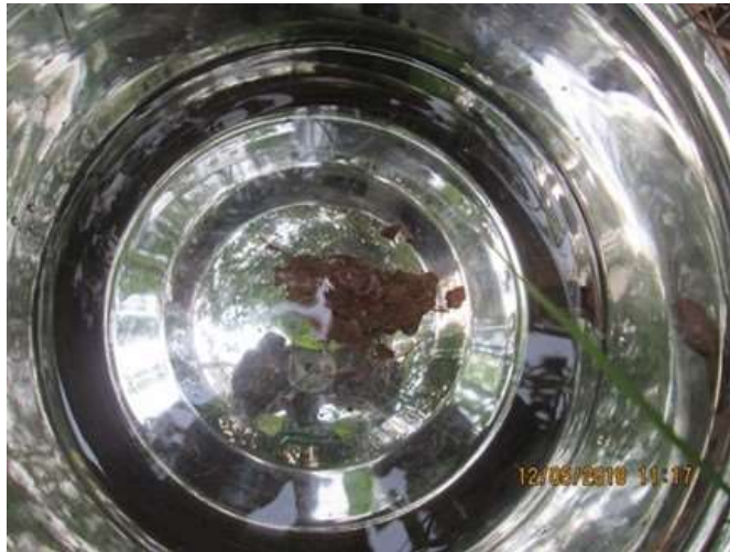
Figure 41 - Start of Slake Test of P2 SS4
