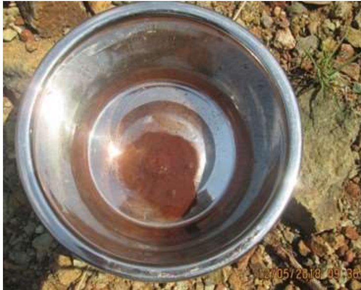
Figure 37 - Start of Slake Test, P7 SS2
