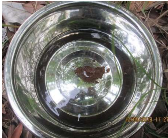
Figure 42 - End of Slake Test of P2 SS4
