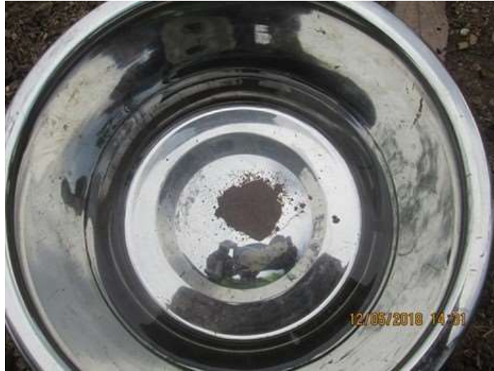
Figure 43 - Start of Slake Test P8 SS5
