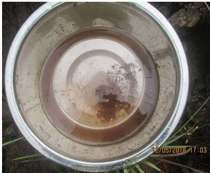
Figure 46 - End of Slake Test P2 SS6
