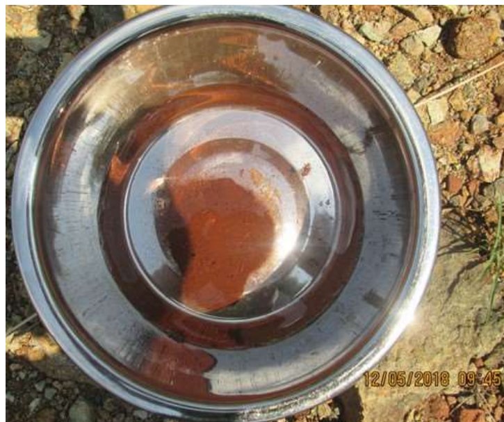
Figure 38 - End of Slake Test, P7 SS2
