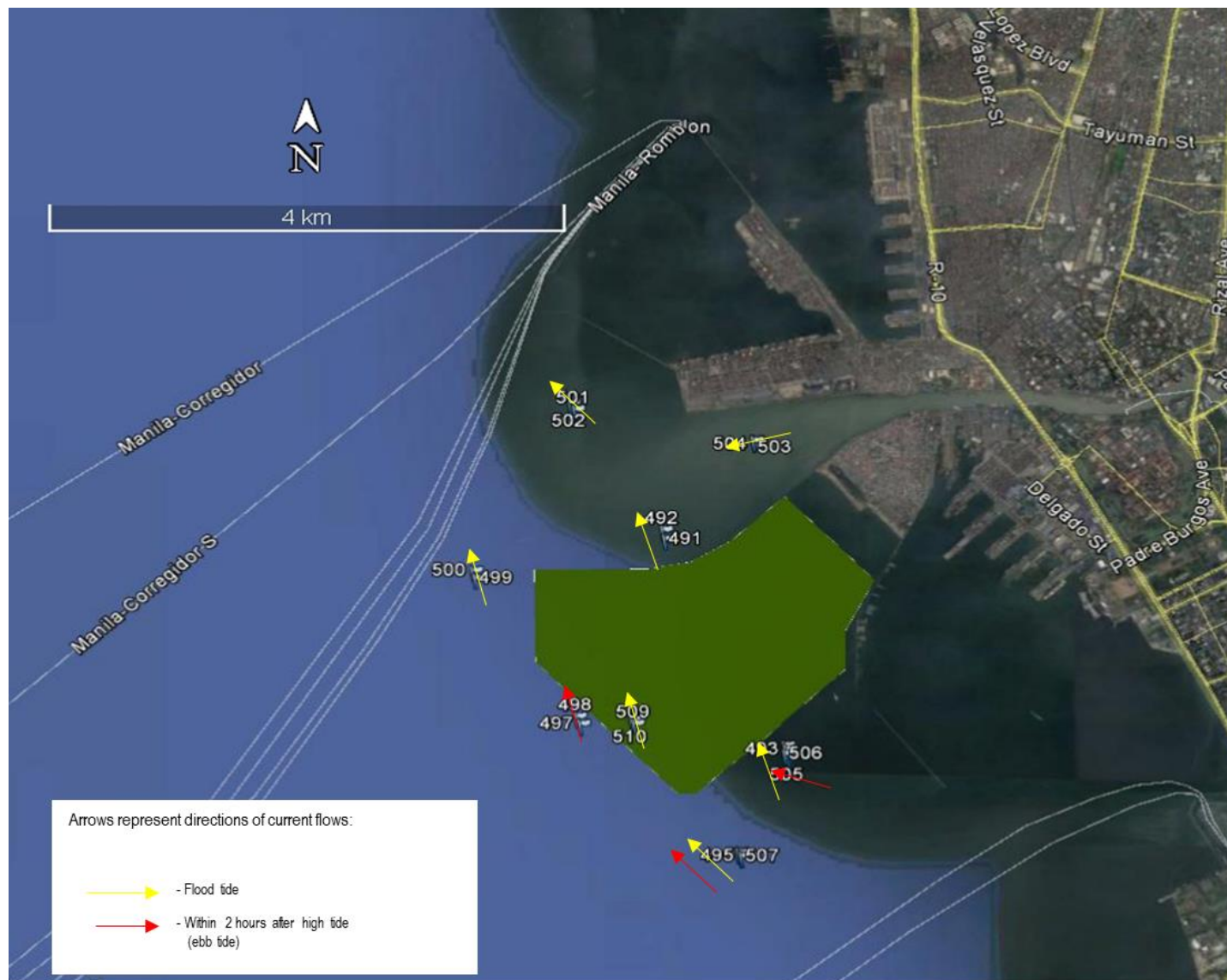
Figure 2-26. Observed current directions during flood tide and within 2 hours after high tide (or ebbing tide) on June 29, 2018
