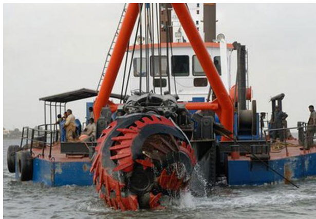
Plate PD-1. A Cutter Dredger
