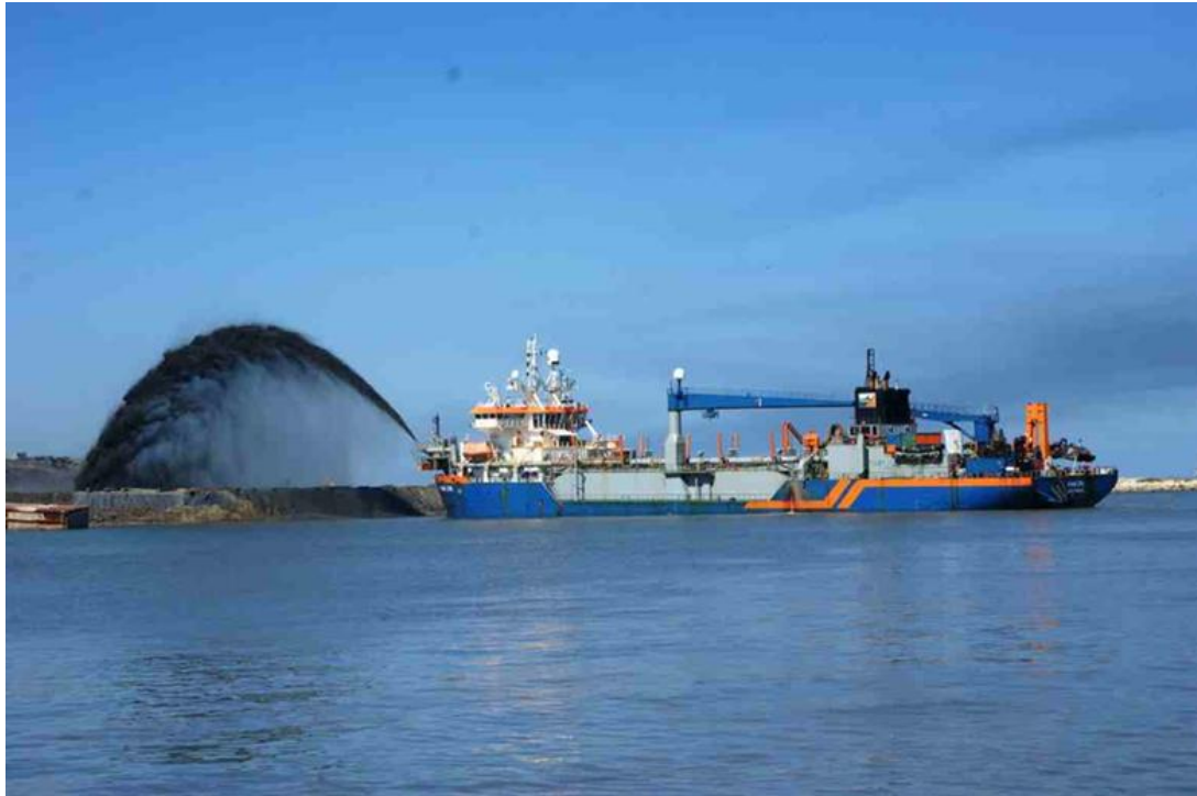
Plate PD-2. A Typical Trailer Suction Header Dredger (TSHD)
