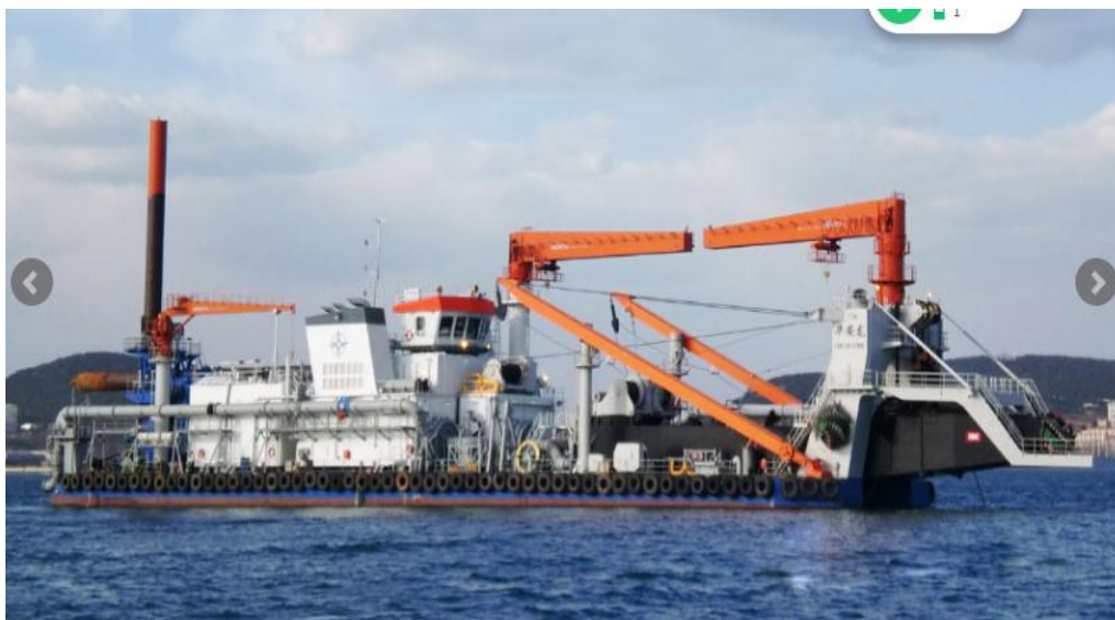
Plate PD-4. An Illustration of a Typical Hydraulic Dredger
