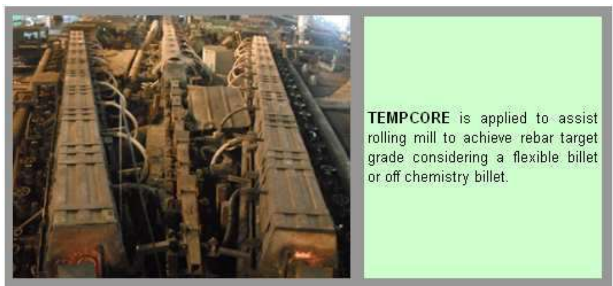
Plate 4: Water Quenching Line / Use of Tempcore
