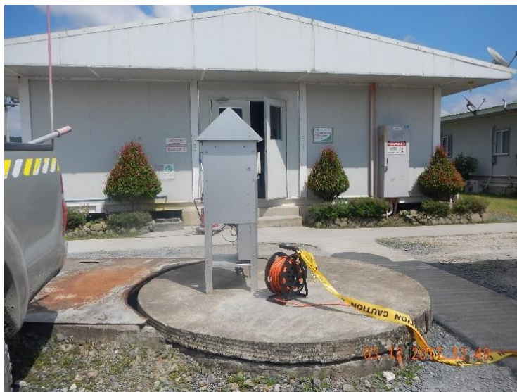
Photo 6-19: High-volume sampler for Total Suspended Particulates (TSP)
