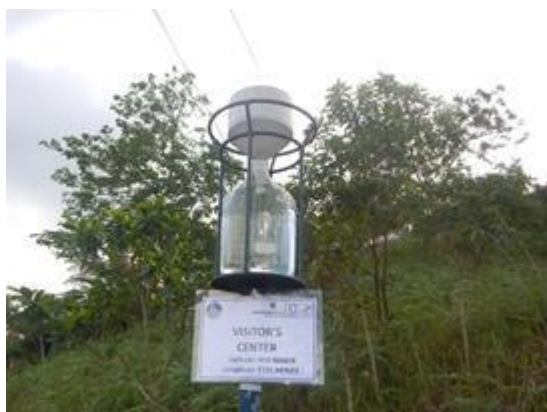
Photo 6-20: Dust Deposition Gauge (DDG)
