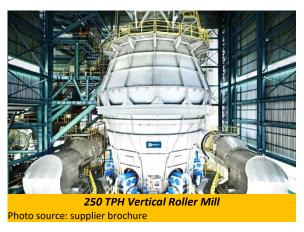
coarse particles are rejected out of the mill and are re-circulated into the mill for re-grinding. The finer particles pass thru the classifier and are carried by the exit gases that will pass thru a bag filter where the finished cement will be separated by the bags and collected at the bottom of the bag filter and subsequently conveyed into the cement silos. There is internal recirculation of the particles that could not pass thru the internal classifier.
