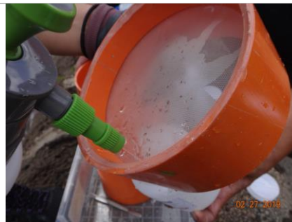
(e) Specimens are transferred into sampling bottles.
