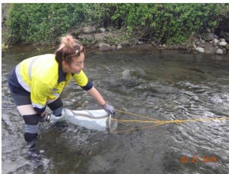
(a) Plankton nets are dragged against stream flow to collect samples.
