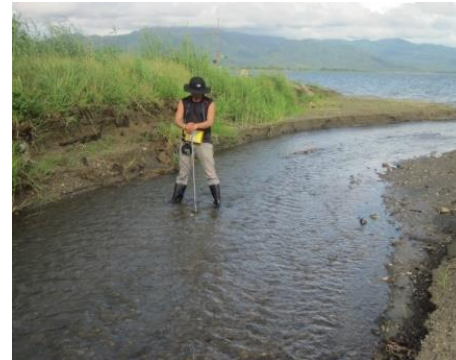
Plate 2.2.2-7 Stream velocity measurement at SW10-AO-AR using the Valeport Ltd® "Braystroke" meter
