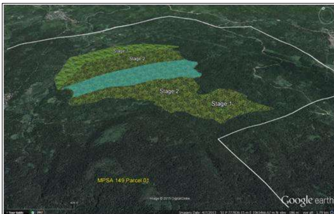
Figure 6.2-7 Stage 2. By Stage 2 the tailings beach would be shown in the previous figure will be covered with grass to allow the tailings beach to transition into more consolidated ground.
