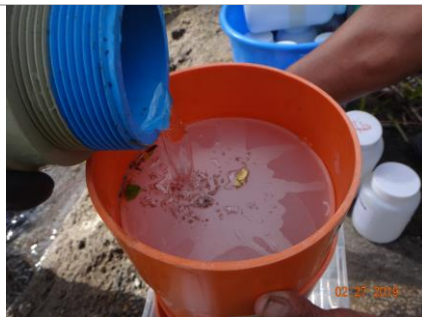
(d) Collected sample is filtered through stackable sieves of 500µm, 220 µm and 120 µm.
