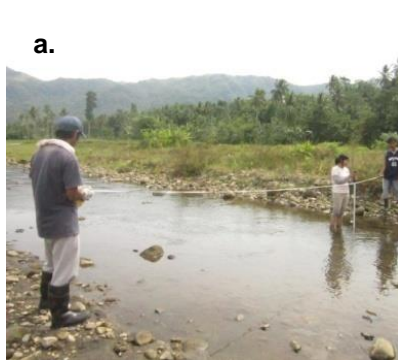
Plate 2.2.2-6 In-situ measurement of stream-width, depth, and velocity using the Global Water® Flow model FP111 current flow meter at Stations (a.) SW3-MG-UPR and (b.) SW17-HA-UP
