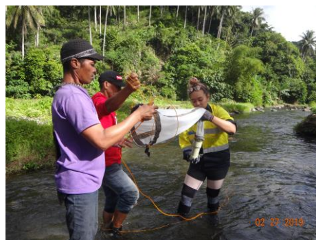
(b) Plankton nets are rinsed to concentrate samples towards the cod end in preparation for transfer into sampling bottles.
