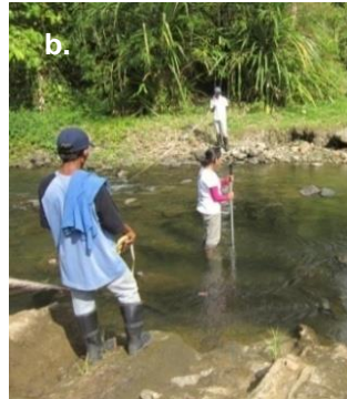
Plate 2.2.2-6 In-situ measurement of stream-width, depth, and velocity using the Global Water® Flow model FP111 current flow meter at Stations (a.) SW3-MG-UPR and (b.) SW17-HA-UP
