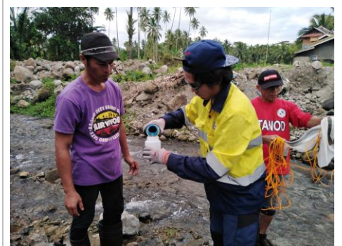
(c) Plankton sample being transferred into sampling bottle, preserved and sealed to be taken to the lab for analysis.
