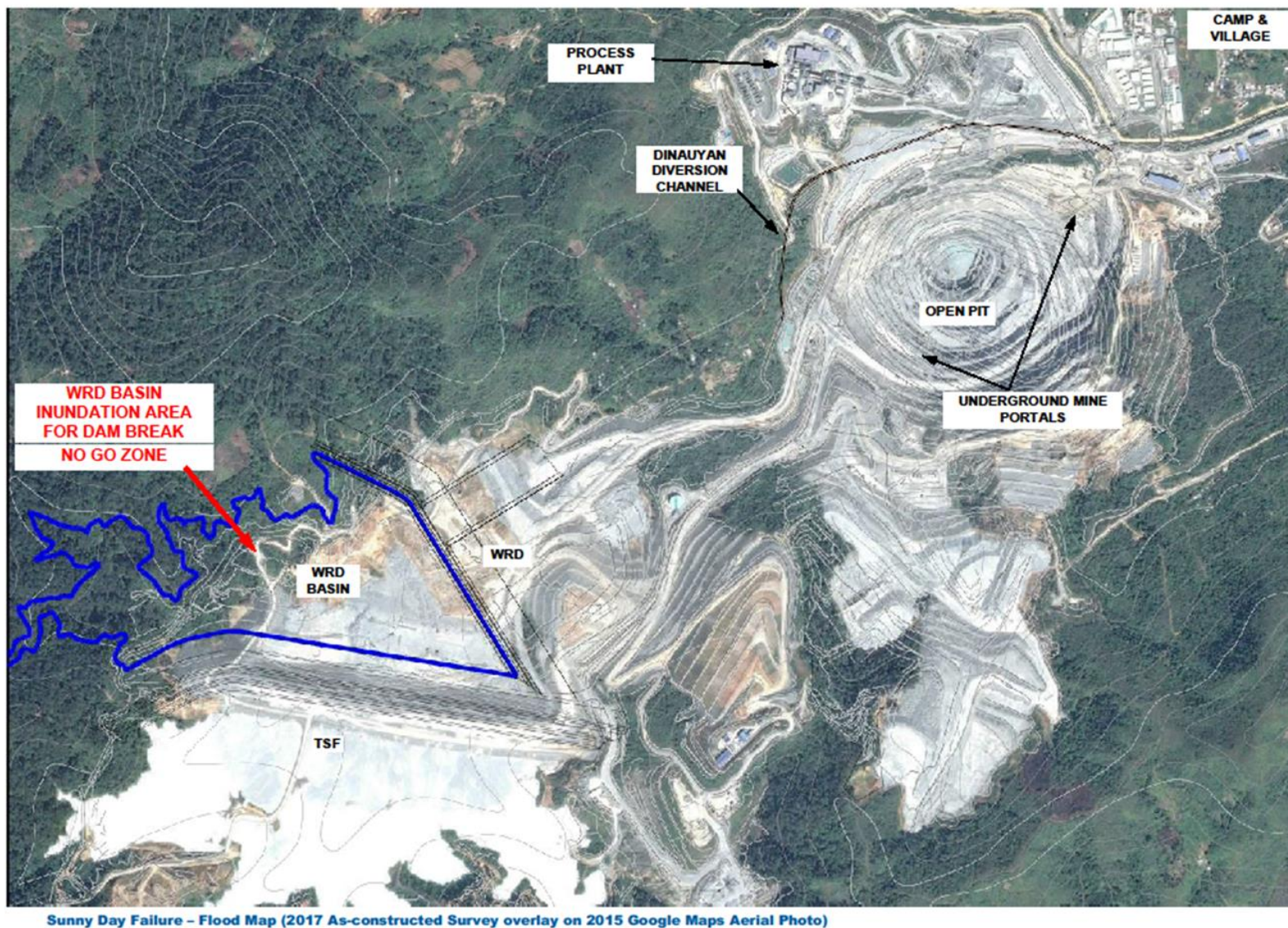
Figure 4-6: Sunny Day Failure – Flood Map
