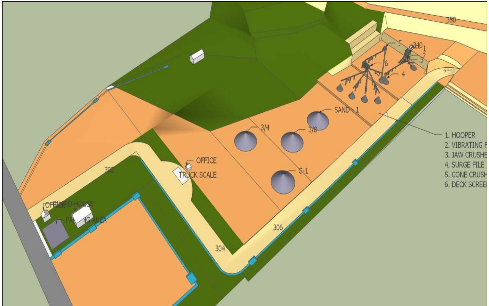
Figure 4: Indicative Project Components Layout
