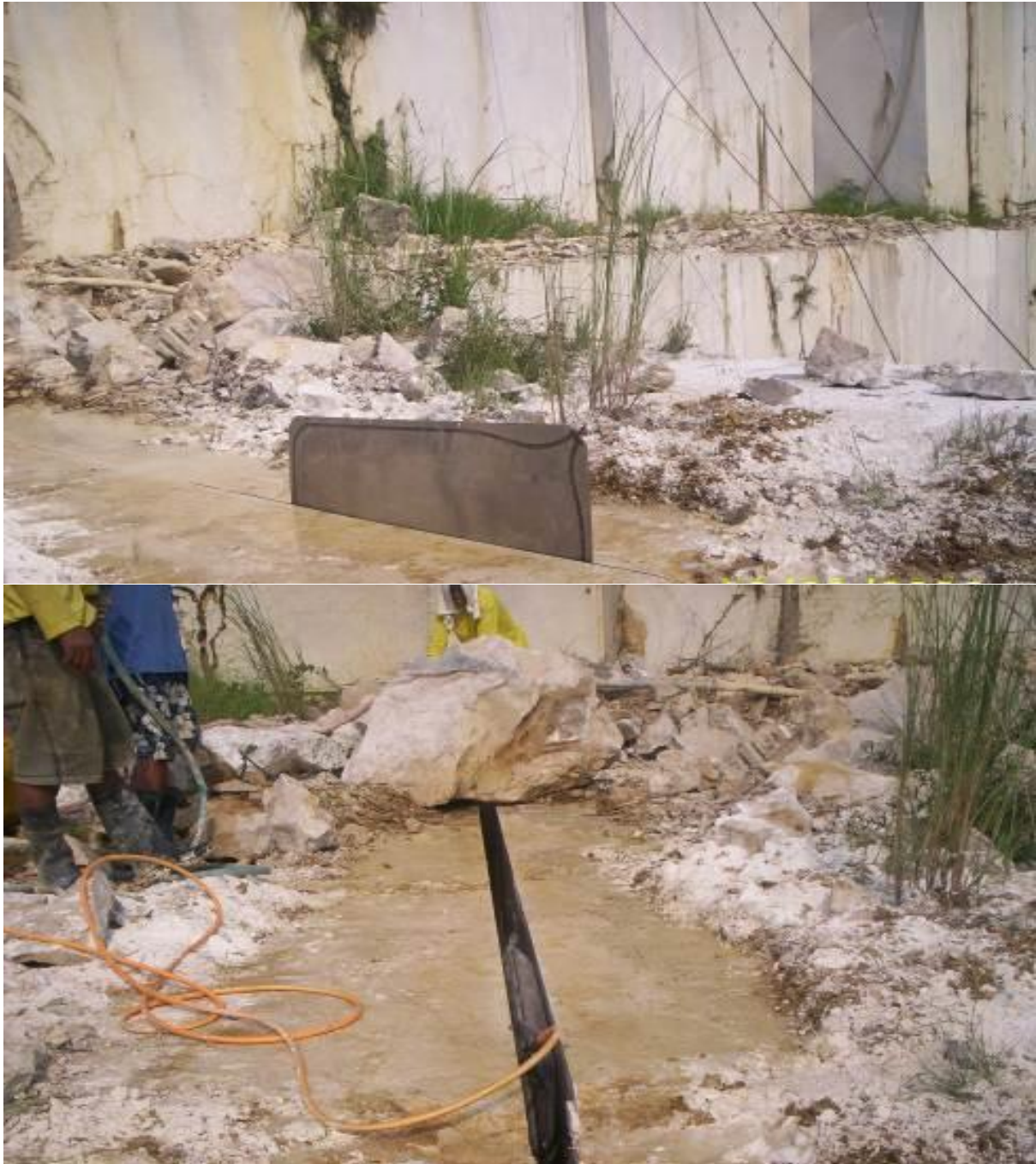
Figure 1-20: Toppling Bancatta Using Hydro Bag
