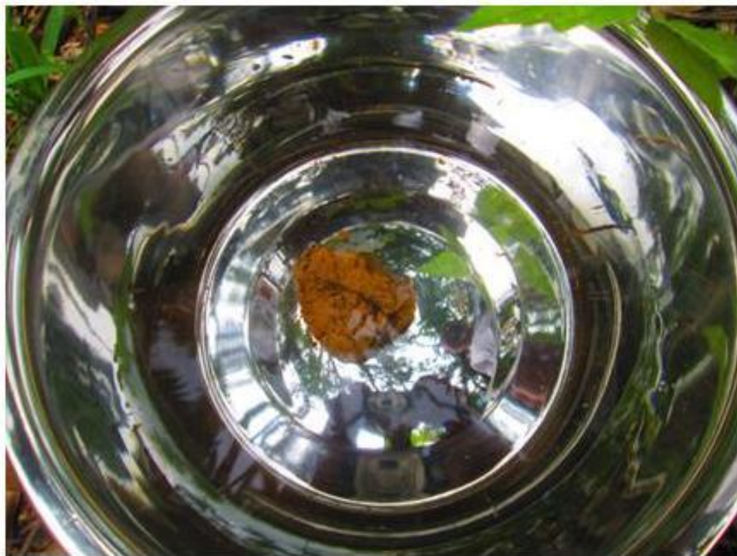
Figure 2-18: Start of Slake Test, Parcel 1
