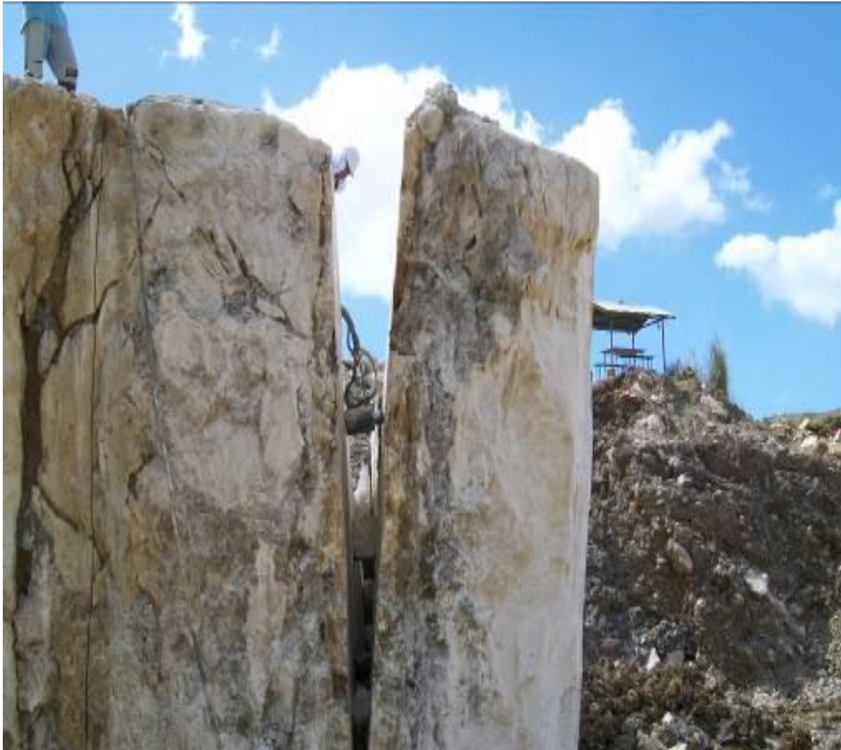
Figure 1-19: Toppling Bancatta Using Titano Jack
