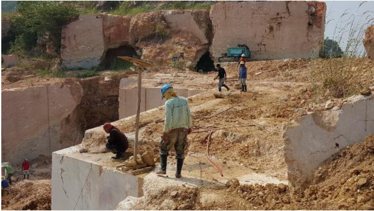
Figure 1-18: Laying out of Wiresaw to cut the Marble into Blocks
