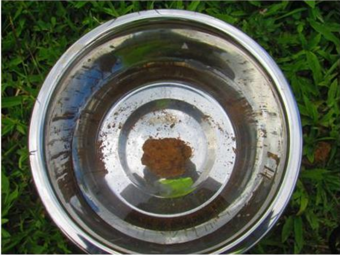
Figure 2-22: Start of Slake Test, Parcel 5
