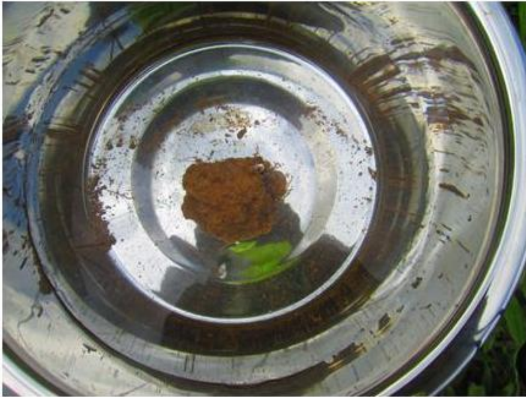
Figure 2-20: Start of Slake Test, Parcel 3
