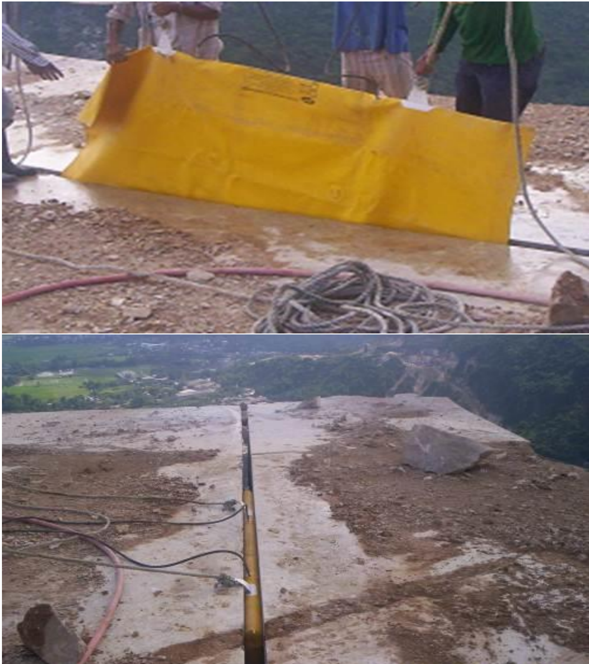
Figure 1-21: Toppling Bancatta Using Airpillow
