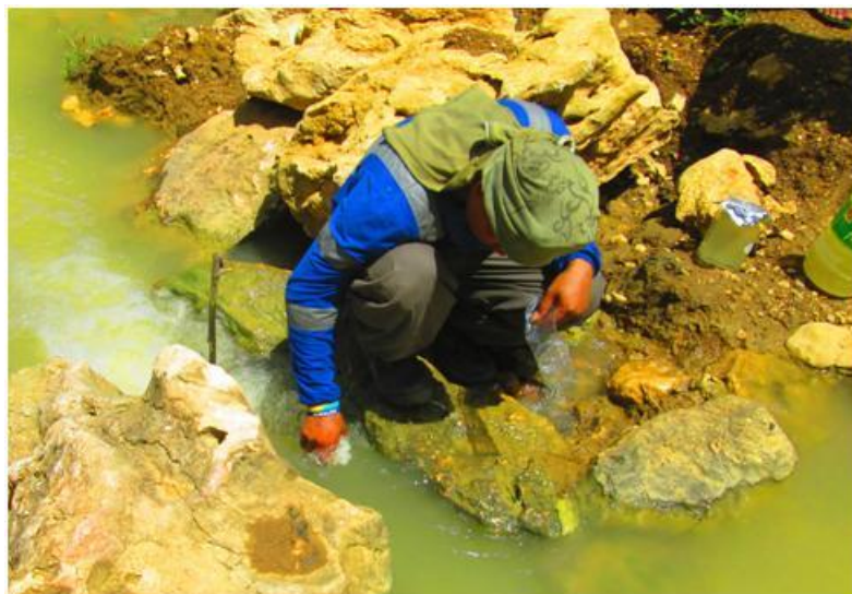
Figure 2-53: Stream Grab Water Sampling
