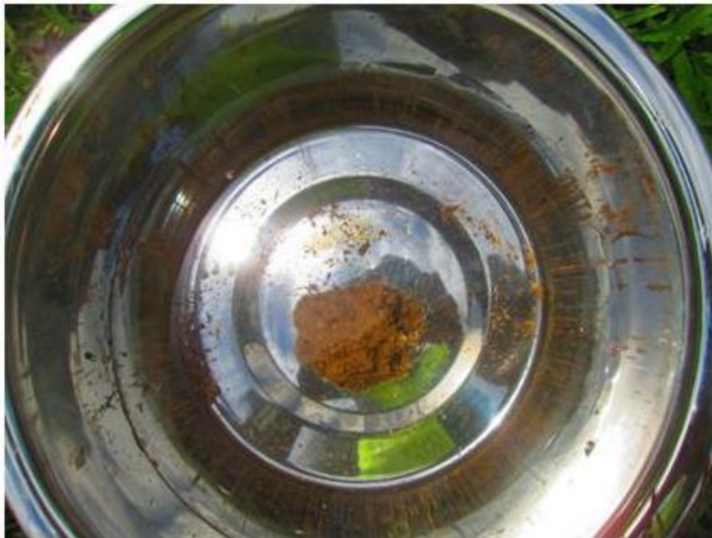
Figure 2-21: 10 Minutes After Slake Test, Parcel 3
