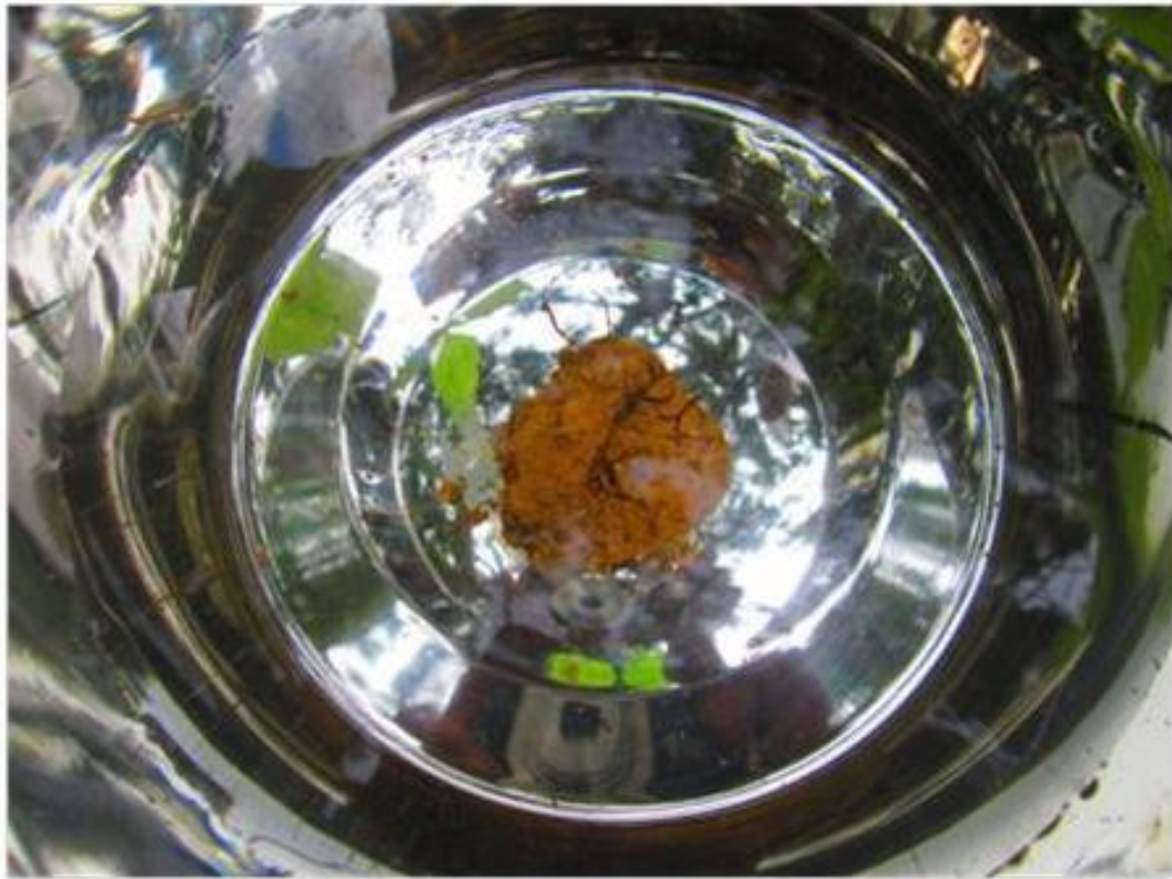
Figure 2-19: 10 Minutes After Slake Test, Parcel 1
