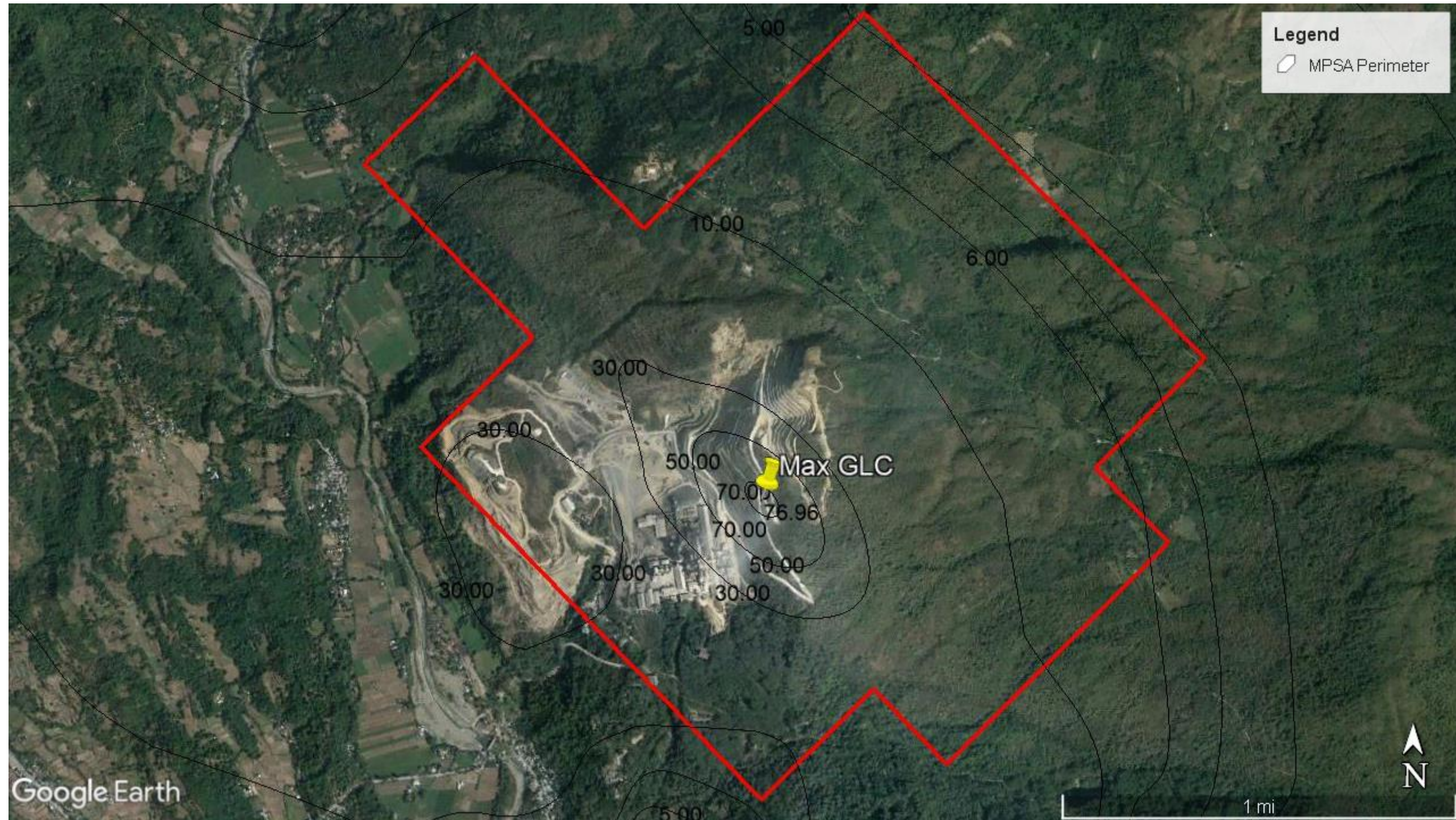
Figure 2-39: Isopleth of the incremental 98 th percentile annual average PM10 concentration ( \mu\text{g}/\text{m}^3 )
