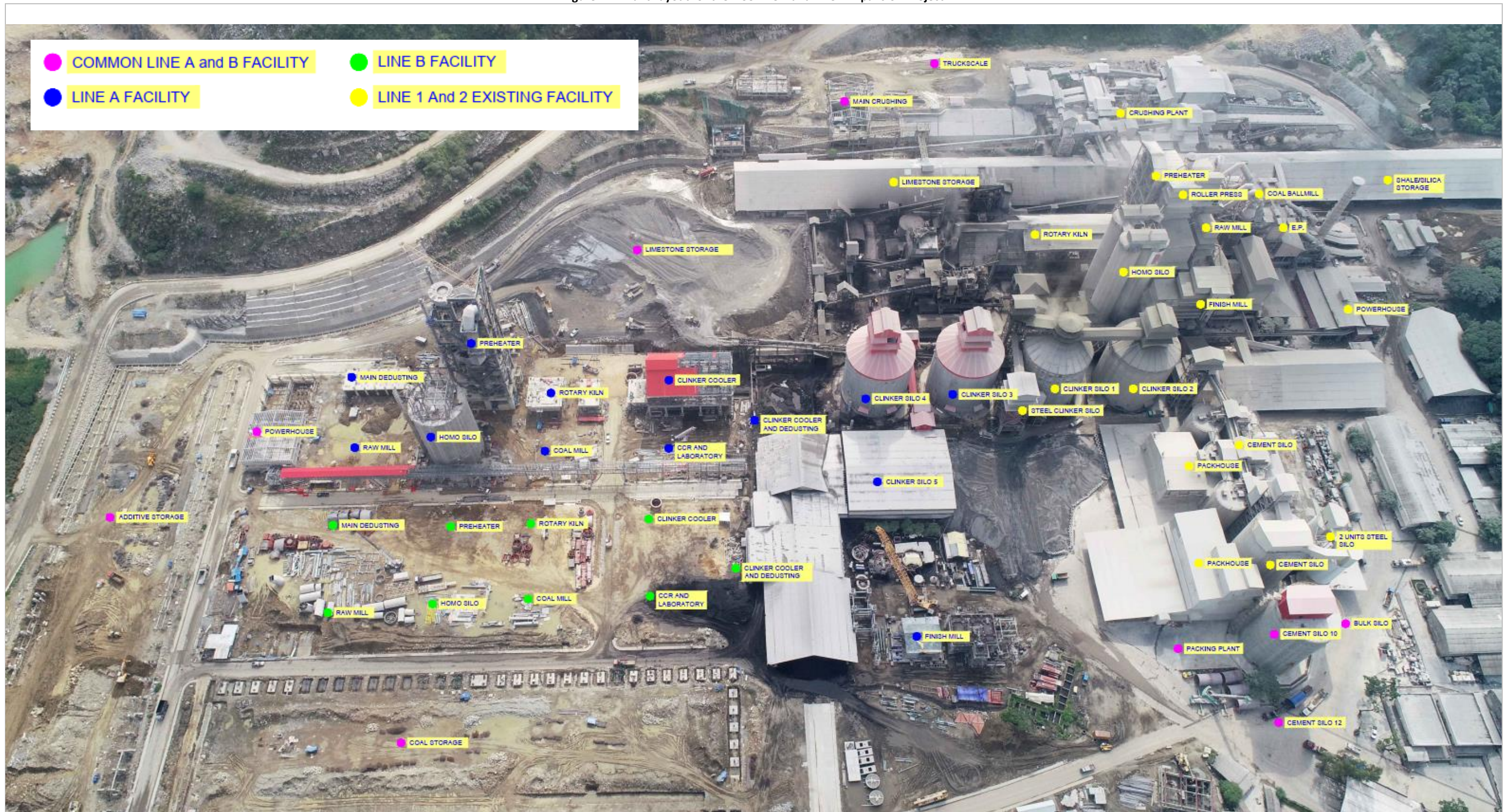
Figure 1-4: Plant Layout for the NCC Line 1 and Line 2 Expansion Project
