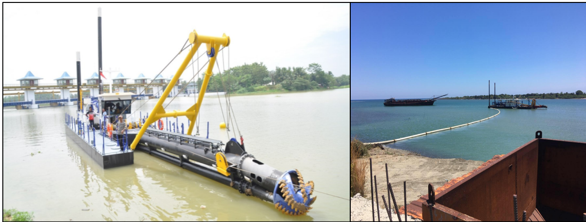
Figure 13: Photos of desilting vessel to be used in the extraction of riverbed materials (left photo) and sand slurry being pumped to the stockpile/processing site on the beach using HDPE pipe (right photo)
