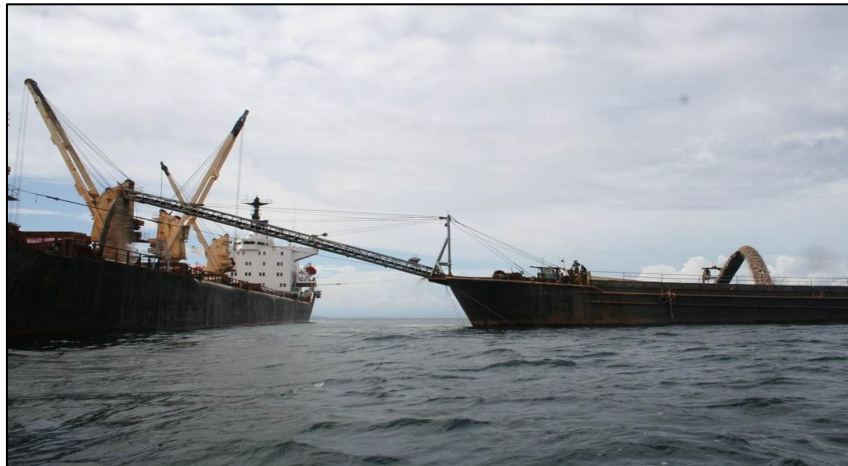
Figure 15: Photo of shuttle conveyor barge discharging the sea sand/processed river sand into the conveyor trans-shipment barge which then uploads the sand onto the ocean vessel
