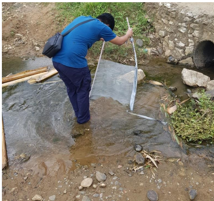
Plate 8 - Benthic macroinvertebrates collection using rectangular kick net
