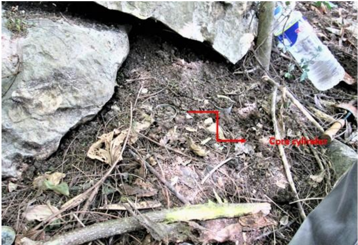
Figure 22 - Soil sampling for Bulk Density Using Stainless steel cores
