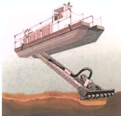
Plate A.1. An Illustration of a Typical Hydraulic Dredger
