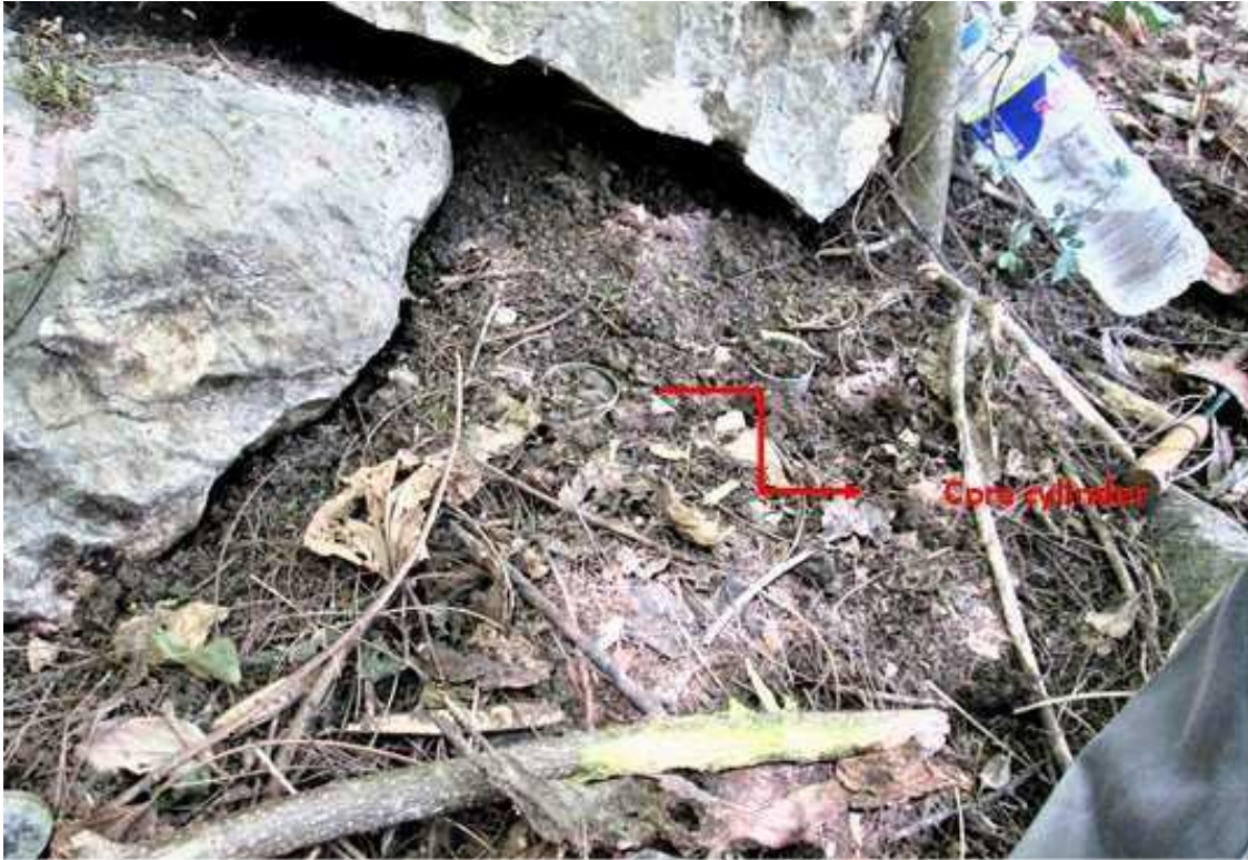
Figure 24 - Soil sampling for Bulk Density Using Stainless steel cores
