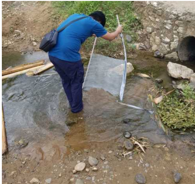
Plate 8 - Benthic macroinvertebrates collection using rectangular kick net
