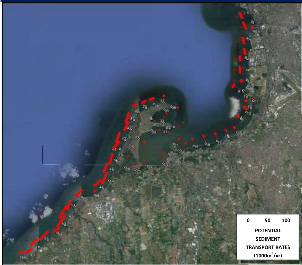
Figure 2.2-95 Directions and Magnitudes of Annual Net Longshore Transport Q_t for Modified Conditions
