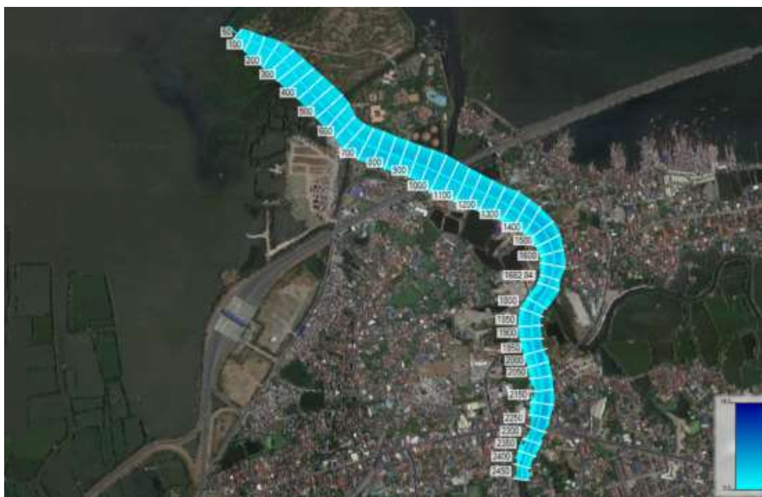
Figure 2.2-16 Inundation map of Imus River for 10-yr Return Period (based on highest historical water level at Manila South Tide Station)
