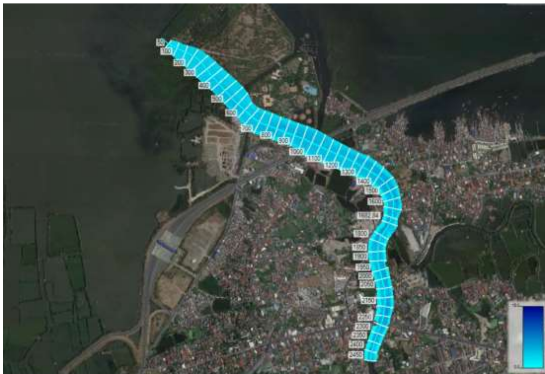
Figure 2.2-18 Inundation map of Imus River for 50-yr Return Period (based on highest historical water level at Manila South Tide Station)
