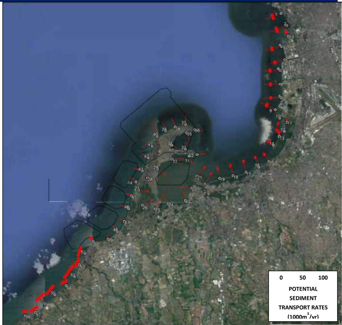
Figure 2.2-96 Directions and Magnitudes of Annual Gross Longshore Transport Q_t for Modified Conditions
