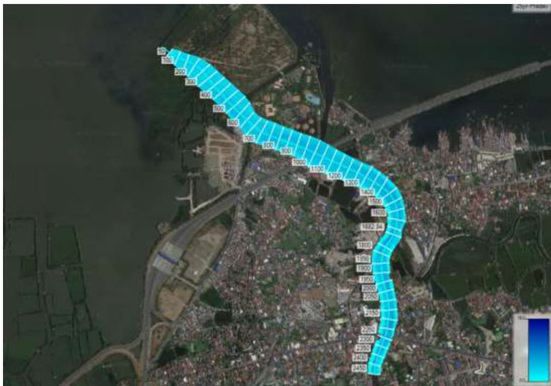
Figure 2.2-22 Inundation map of Imus River for 25-yr Return Period (Pre-development and Post-development Condition)
