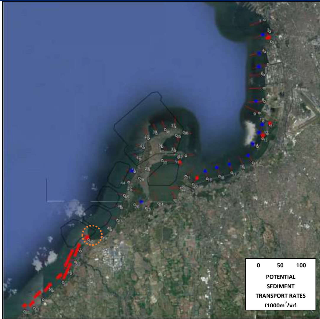
Figure 2.2-94 Directions and Magnitudes of Annual Net Longshore Transport Q_n for Modified Conditions
