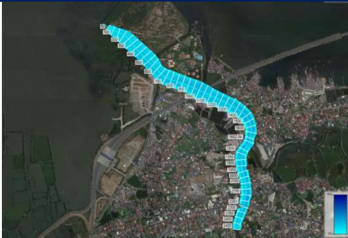
Figure 2.2-17 Inundation map of Imus River for 25-yr Return Period (based on highest historical water level at Manila South Tide Station)
