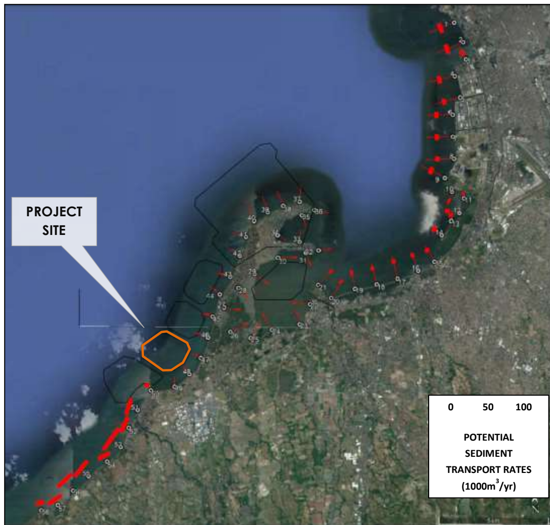
Figure 2.2-90. Directions and magnitudes of annual gross longshore transport Q_t for Modified Conditions
