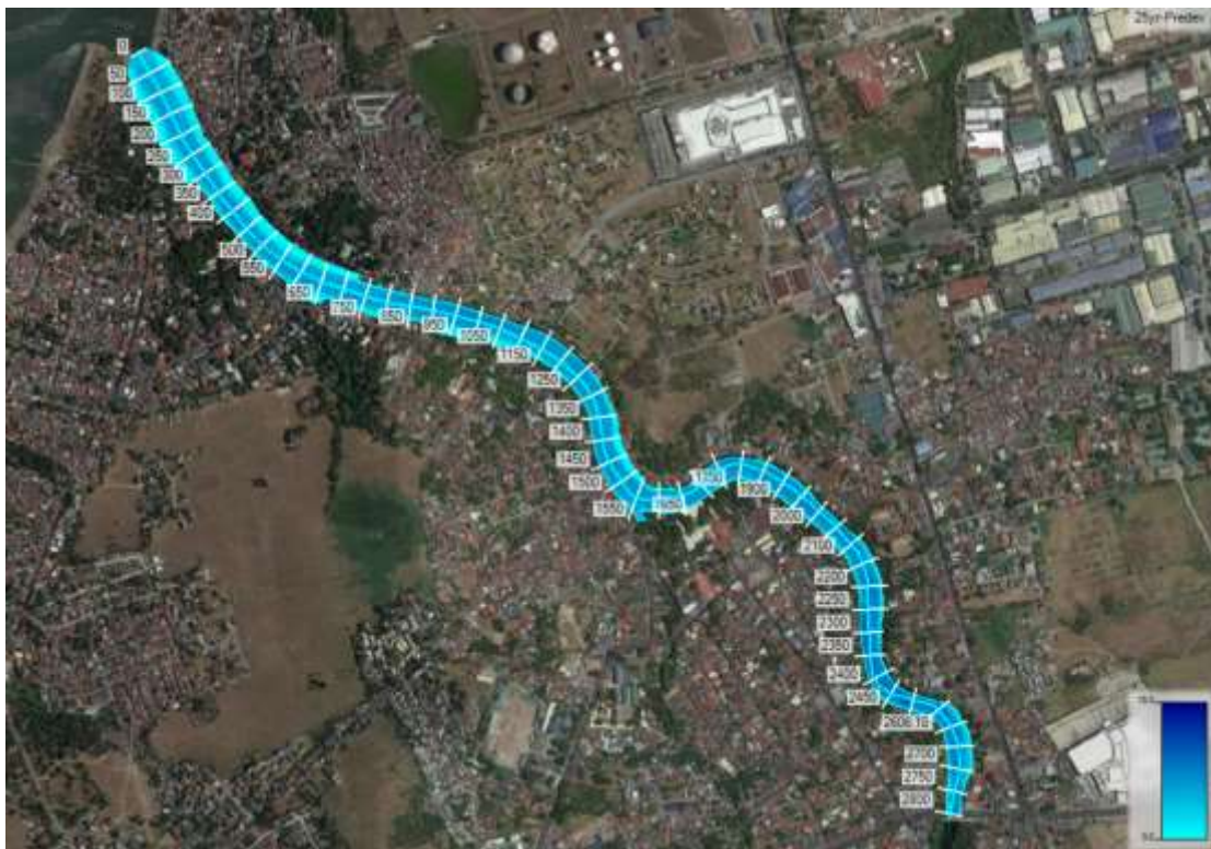
Figure 2.2-29. Inundation Map of Cañas River for 25-yr Return Period (Pre-development and Post-development Condition)
