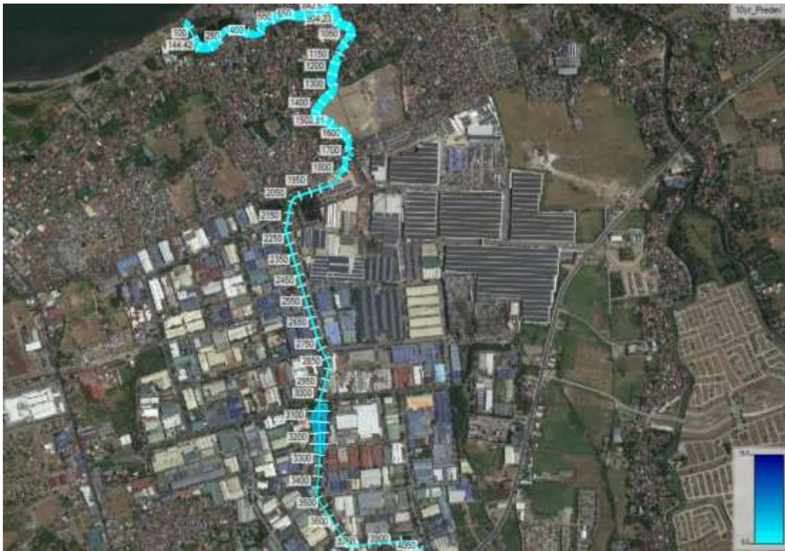
Figure 2.2-17. Inundation Map of Maalimango River for 10-yr Return Period (Pre-development and Post-development Condition)
