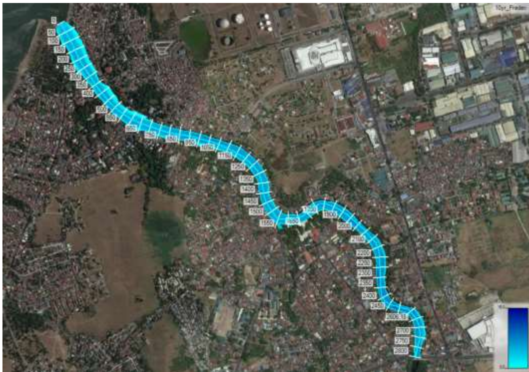
Figure 2.2-24. Inundation Map of Cañas River for 10-yr Return Period (based on highest historical water level at Manila South Tide Station)
