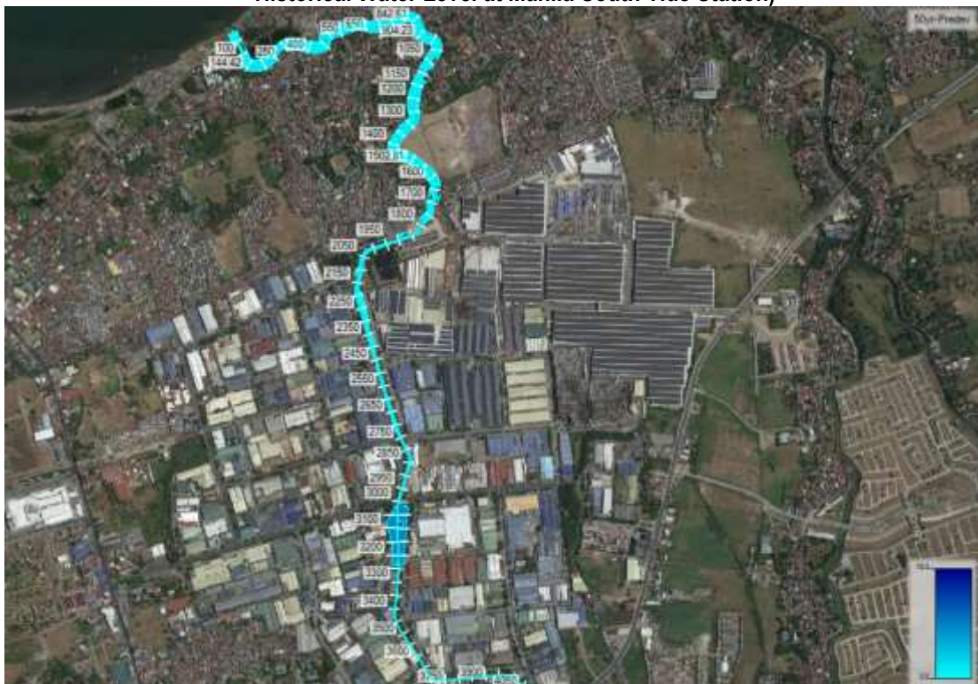
Figure 2.2-14. Inundation Map of Maalimango River for 50-yr Return Period (based on Highest Historical Water Level at Manila South Tide Station)
