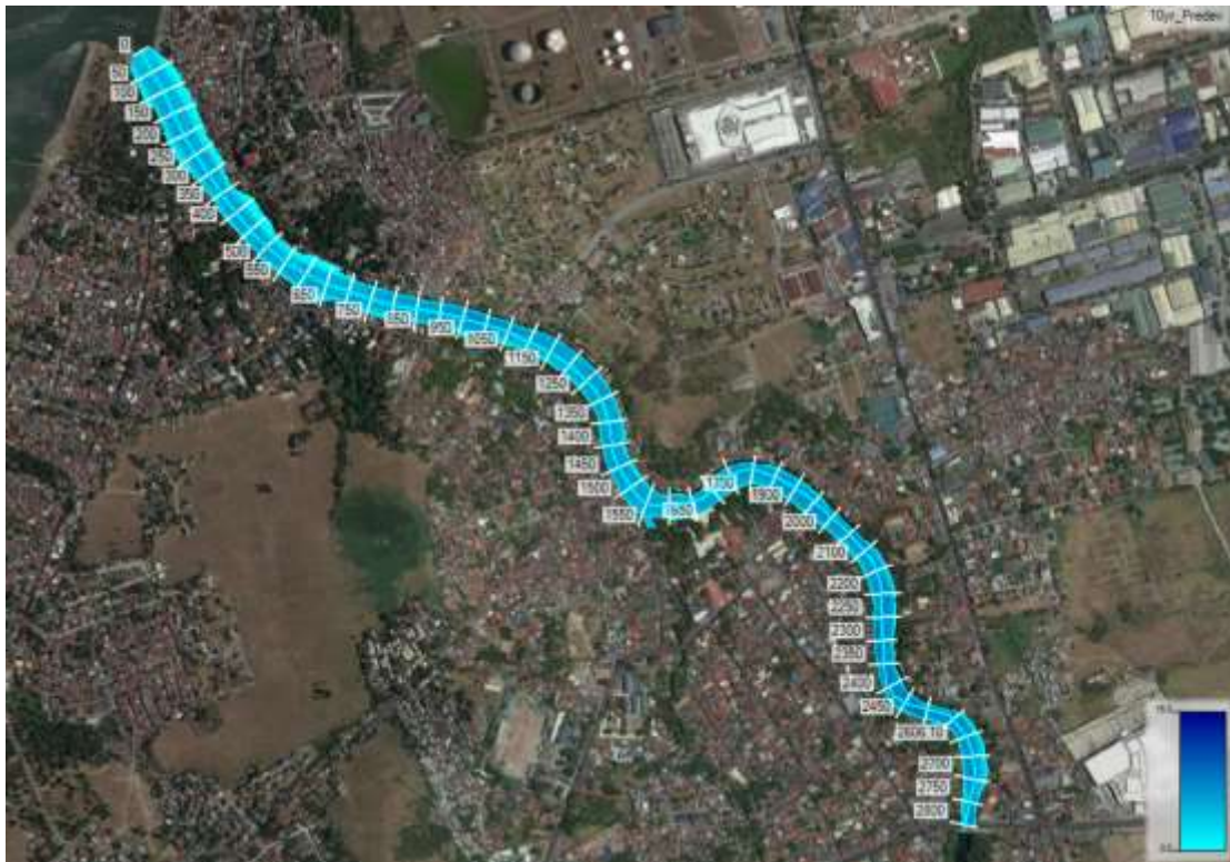
Figure 2.2-28. Inundation Map of Cañas River for 10-yr Return Period (Pre-development and Post-development Condition)
