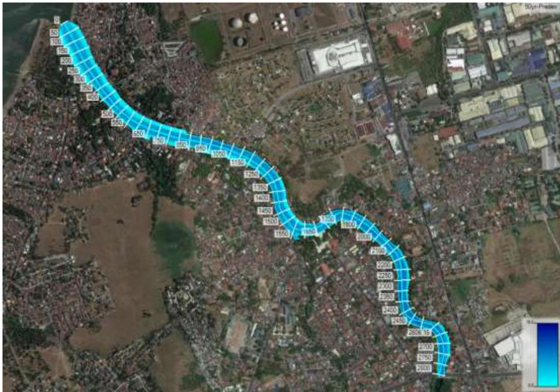
Figure 2.2-30. Inundation Map of Cañas River for 50-yr Return Period (Pre-development and Post-development Condition)
