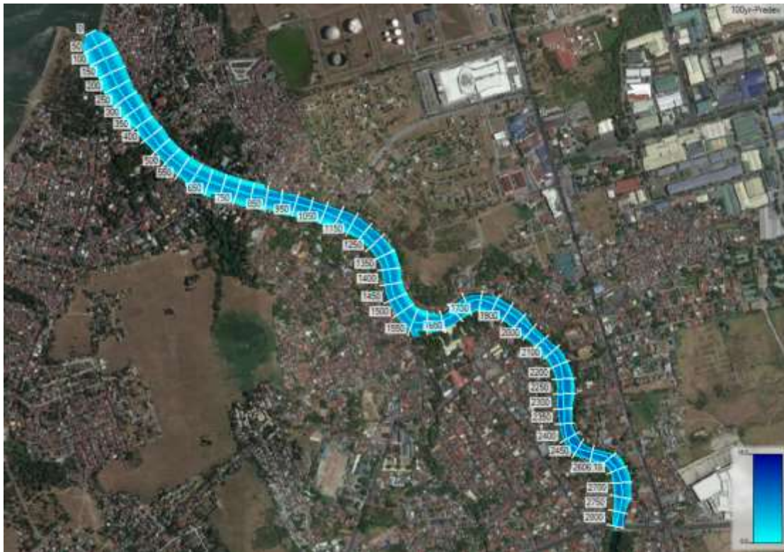
Figure 2.2-27. Inundation Map of Cañas River for 100-yr Return Period (based on highest historical water level at Manila South Tide Station)
