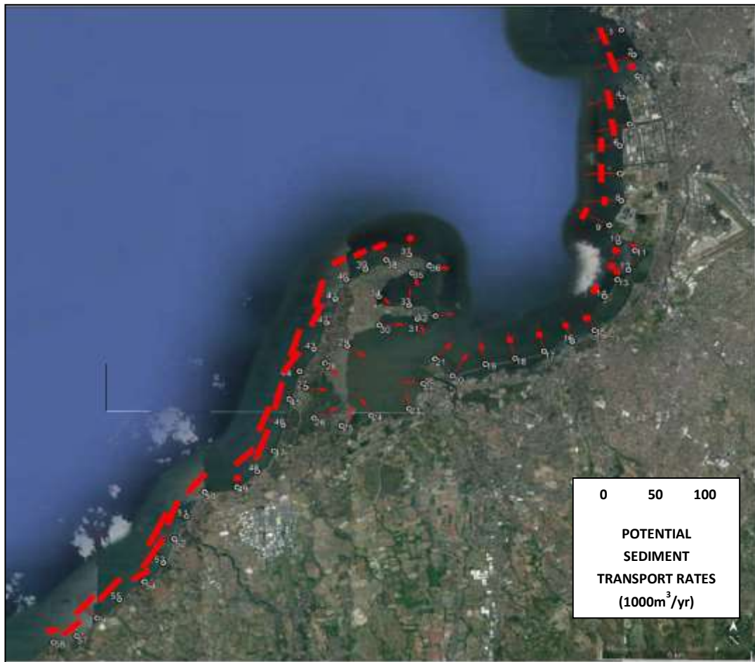
Figure 2.2-89. Directions and magnitudes of annual gross longshore transport Q_t for Baseline Condition
