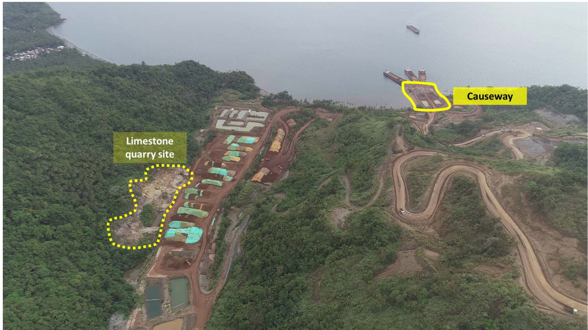
Figure 12 – Limestone quarry site. Payong-payong limestone was used for the construction of the existing causeway for nickel laterite operation.
