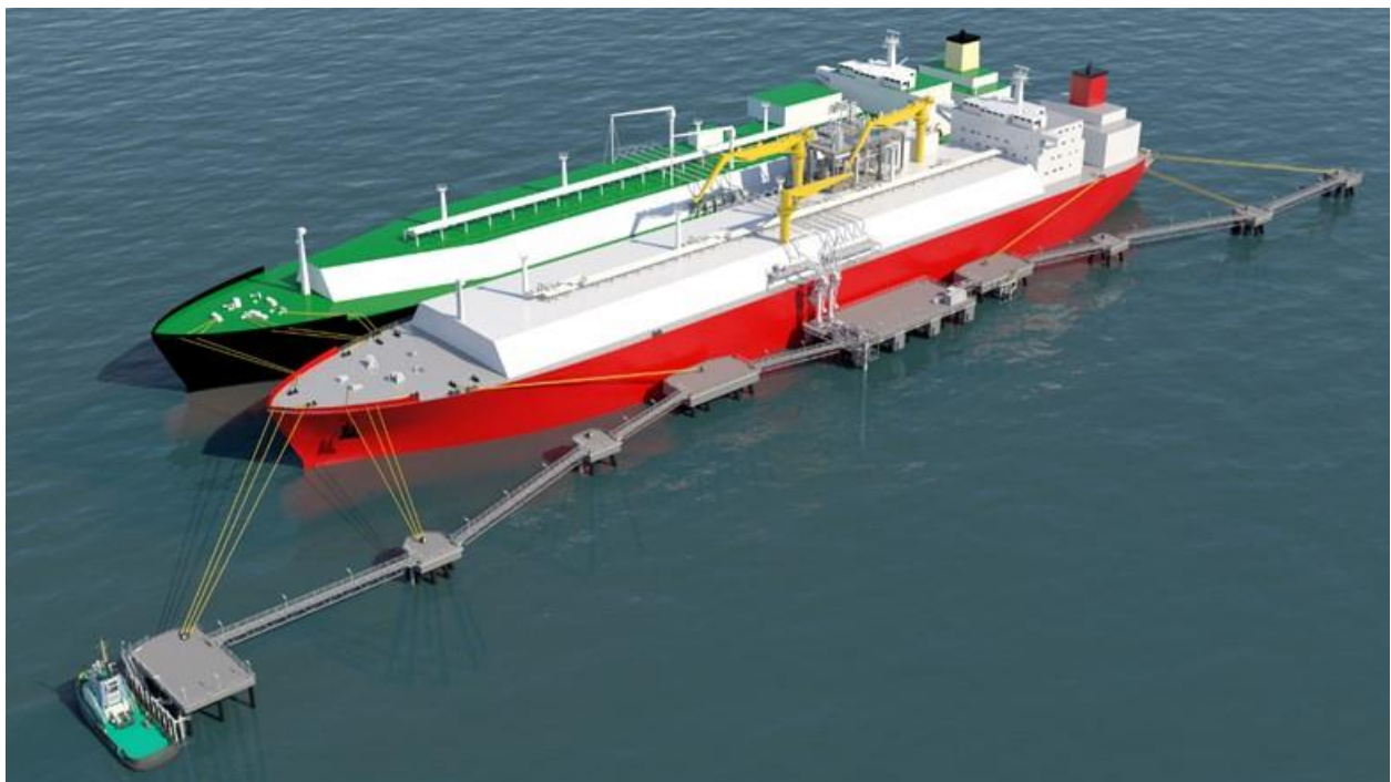
Figure 17 3D rendition of LNG carrier loading into FSRU
