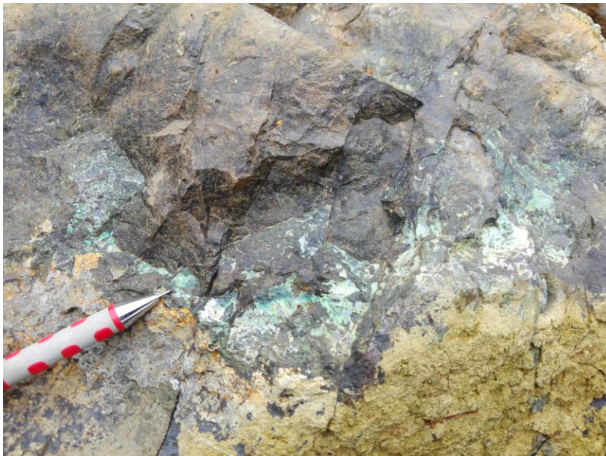
Photo 2. Fracture-fill nickel sulphide garnierite in saprolite in Causwagan open pit.
