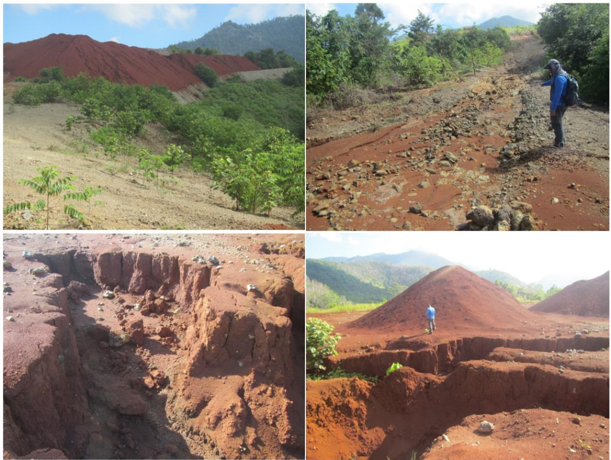
Figure 2.1-42. Photos showing active erosion in the project area and vicinity. Clockwise from top: Laterite stockpile at the mine site in Causwagan block affected by rill erosion, no erosion control measures are present; eroded access road to Causwagan mine site, no drainage canals;
