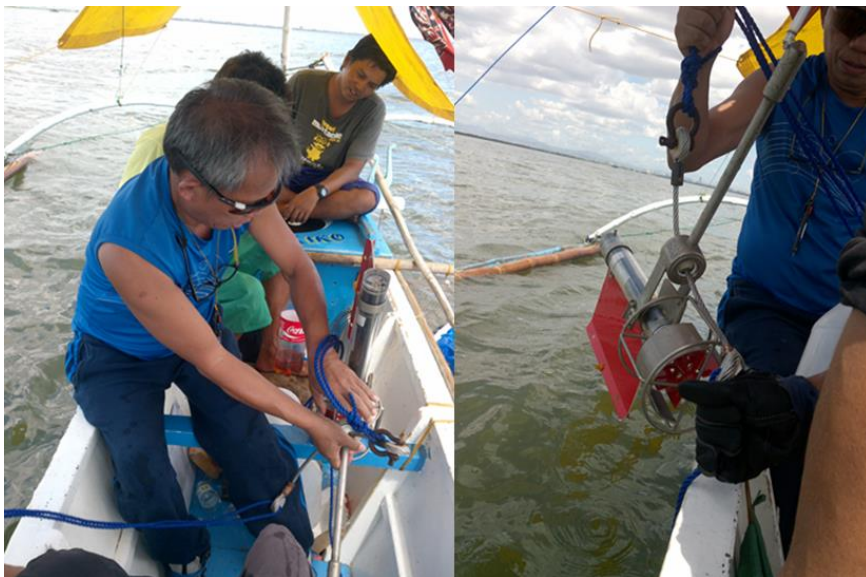
Plate 2-2 An SD 6000 current meter used by Team 1 to measure continuous currents
