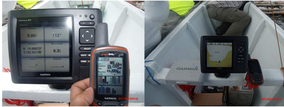
Plate 2-4 GPSMap64S and Garmin Echomap Chirp 52DV used by Team 2 for determination of locations. Garmin Echomap for depth sounding and water temperature measurements
