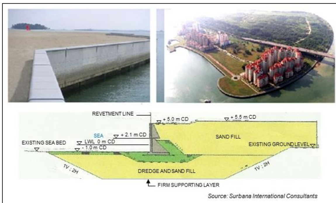
Figure 1-3 Vertical Seawall used in the Tanjong Rhu Reclamation and Southern Island Reclamation in Singapore
