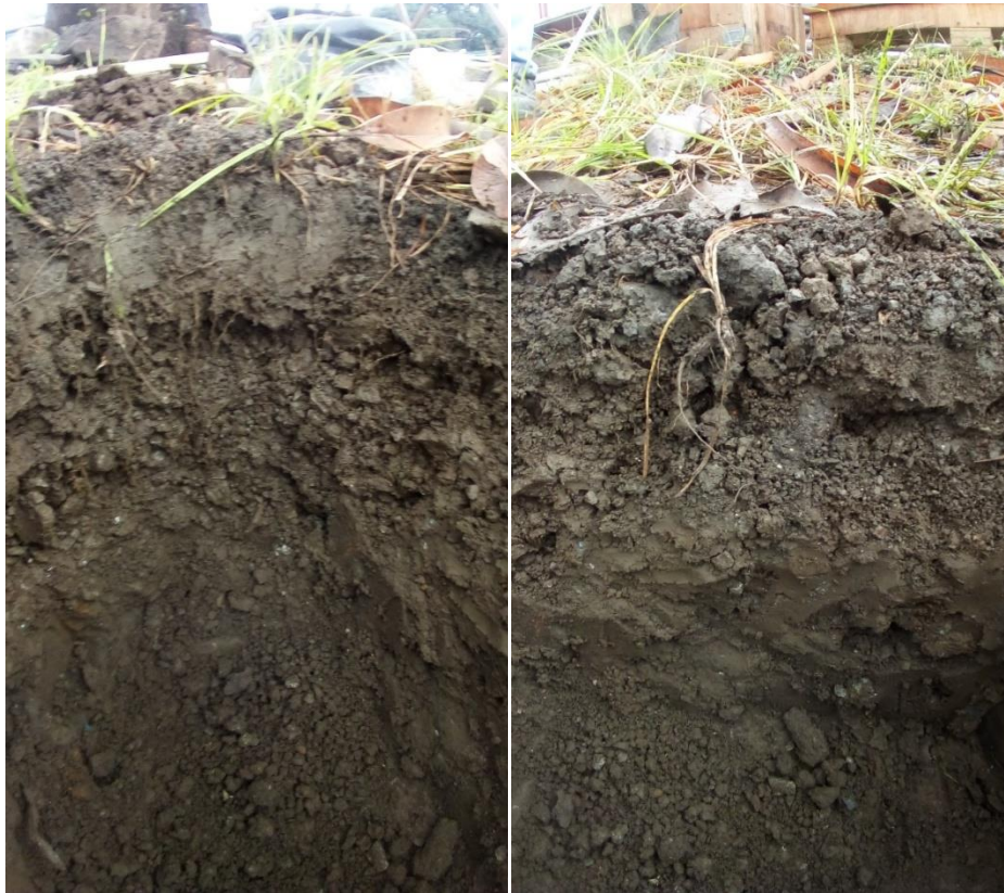
Photo 2.2.1.2a1: Subsoil Profile of TP 1 consisting of gravel to pebble size andesitic material associated with silty soil
