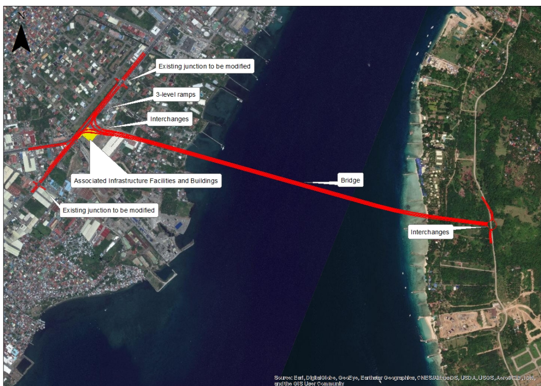
Preliminary Project Components Layout
