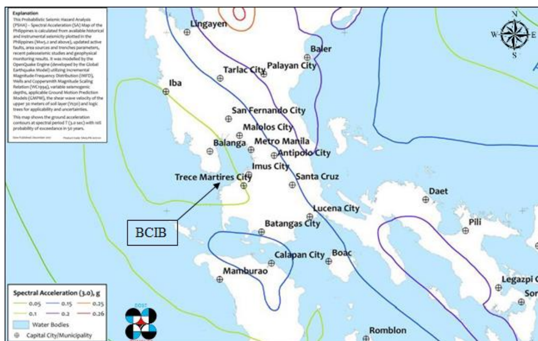
Figure 2.41 Extract of the spectral acceleration map of the Philippine by PHIVOLCS SA (3.0 seconds) at 500-year return period on stiff soil
