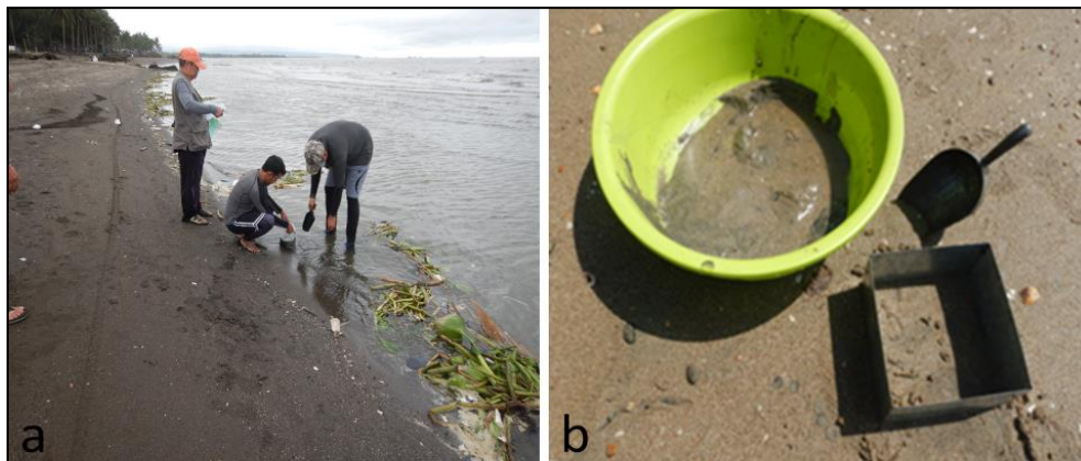
Plate 6 Intertidal benthos sampling at the bridge shore approach in Timalan Concepcion, Naic (a), and a metal frame covering an area of 0.0225 \text{ m}^2 used to collect intertidal infaunal benthos samples (b)
