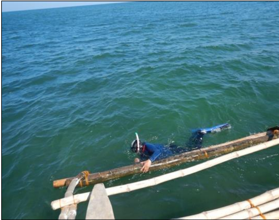
Plate 9 Modified manta tow survey technique wherein a snorkeler is being towed by a motorized outrigger boat along the proposed bridge alignment in Barangay Alas-asin (Mariveles)
