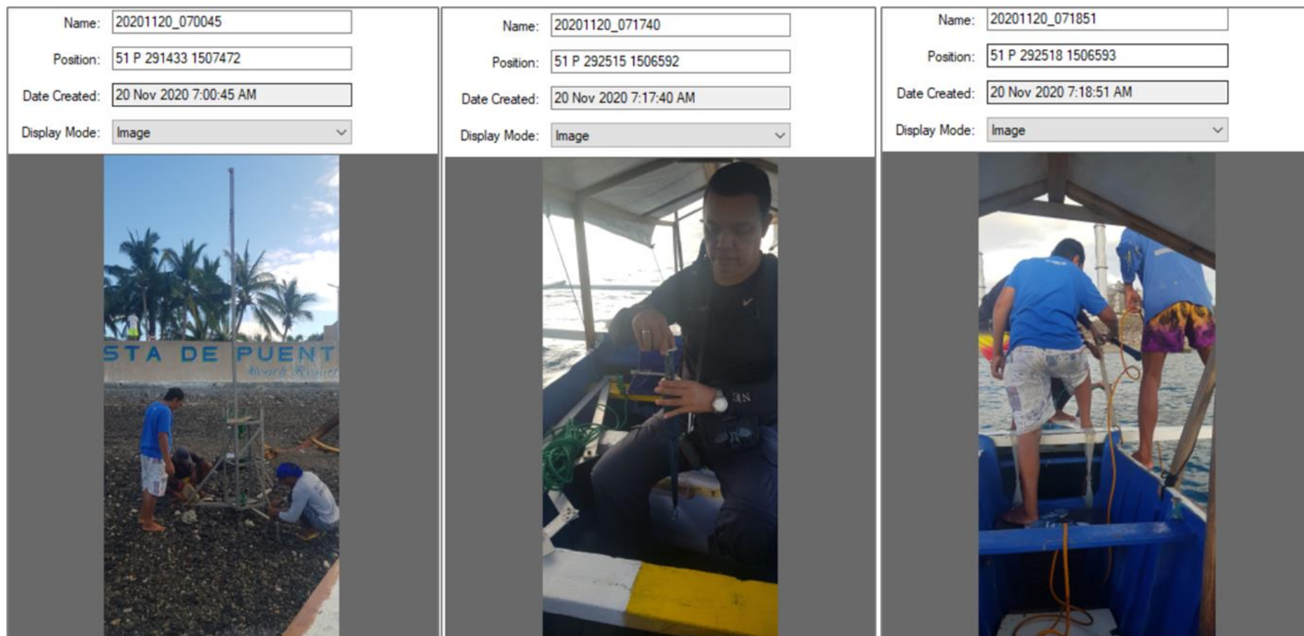
Plate 2-3. Preparation of the aluminum/stainless steel frame (left) and the Marotte HS Tilt Current Meter (middle) and deployment of the Marotte current meter placed on top of the aluminum/stainless steel frame
