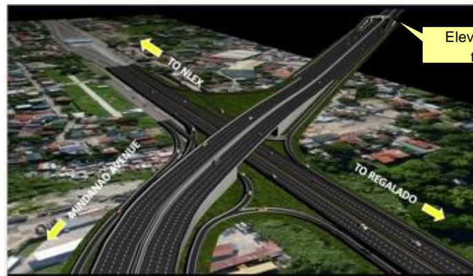
Option 2: On-grade Diamond Type with Elevated U-turn for Mindanao-NLEX Bound Traffic (Initially Selected Option)
