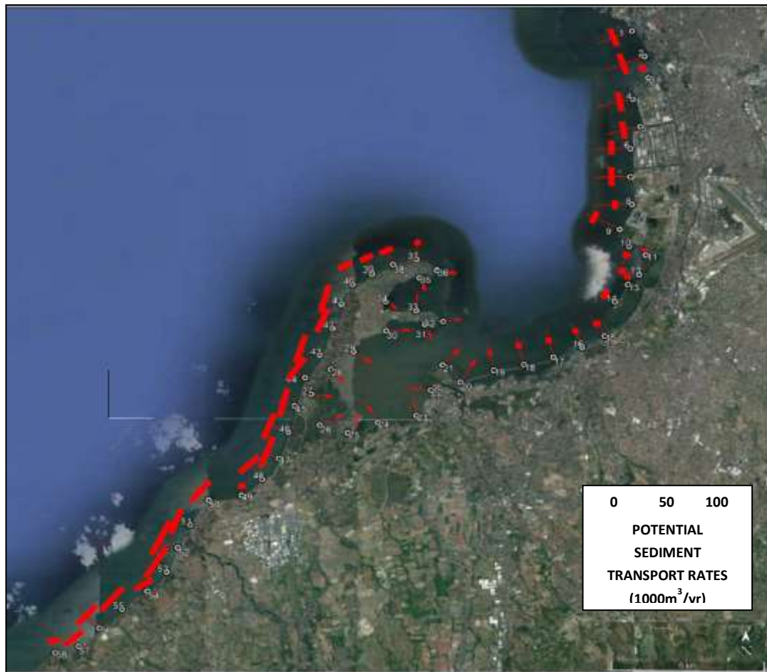
Figure 2.2-87. Directions and magnitudes of annual gross longshore transport Q_t for Baseline Condition
