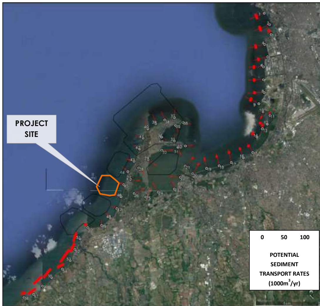
Figure 2.2-88. Directions and magnitudes of annual gross longshore transport Q_t for Modified Conditions
