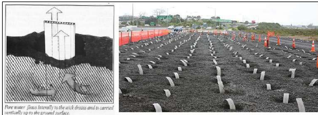
Plate 1-13. Illustration of the Principle of Wick Drains
