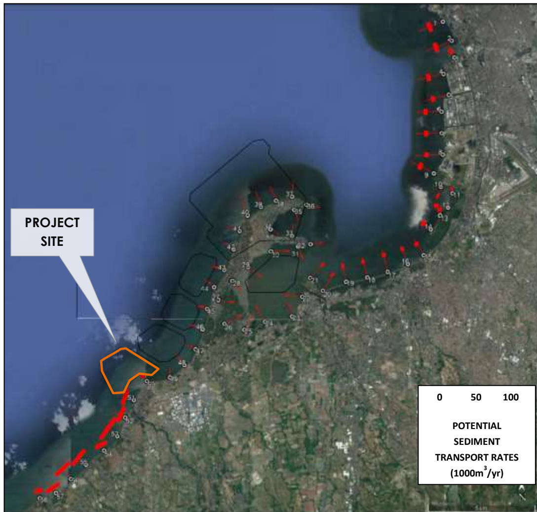
Figure 2.2-86. Directions and magnitudes of annual gross longshore transport Q_t for Modified Conditions
