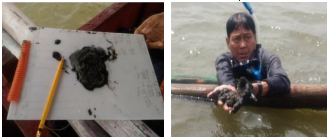
Plate 2.2-9. Muddy sediments and silt-encrusted sand dominate the seabed in the proposed reclamation Island E in Rosario, Cavite.
