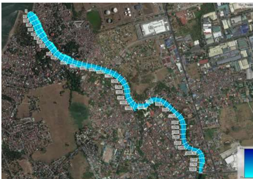
Figure 2.2-22. Inundation Map of Cañas River for 10-yr Return Period (based on highest historical water level at Manila South Tide Station)
