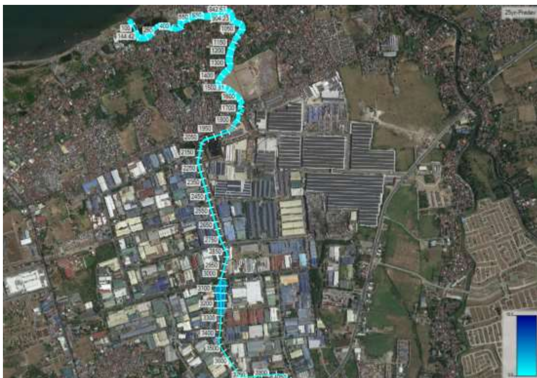
Figure 2.2-11. Inundation Map of Maalimango River for 25-yr Return Period (based on Highest Historical Water Level at Manila South Tide Station)
