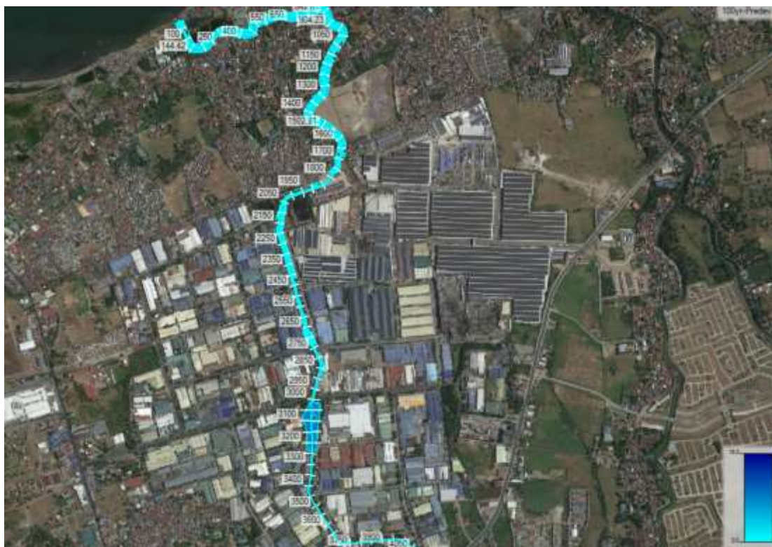
Figure 2.2-13. Inundation Map of Maalimango River for 100-yr Return Period (based on Highest Historical Water Level at Manila South Tide Station)
