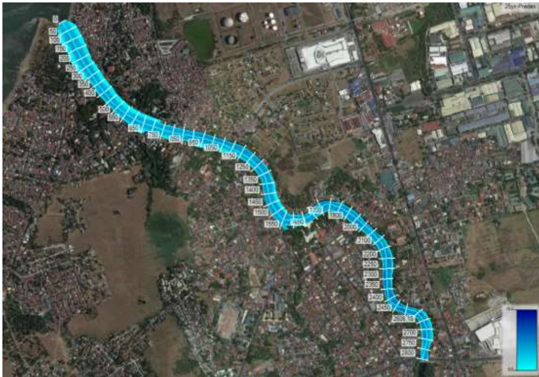
Figure 2.2-23. Inundation Map of Cañas River for 25-yr Return Period (based on highest historical water level at Manila South Tide Station)
