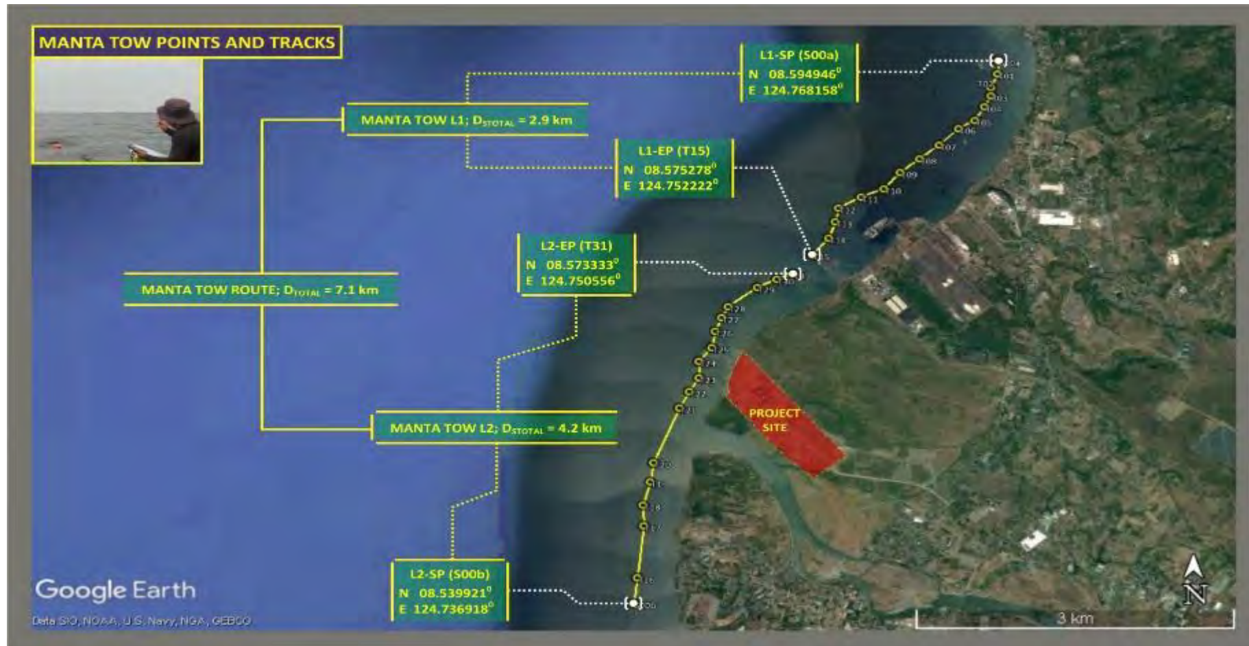
Figure 2.2-62. Manta tow pathways for benthic substrate characterization and location of corals and seagrass resources surveyed during the 2013 marine ecology baseline assessment.
