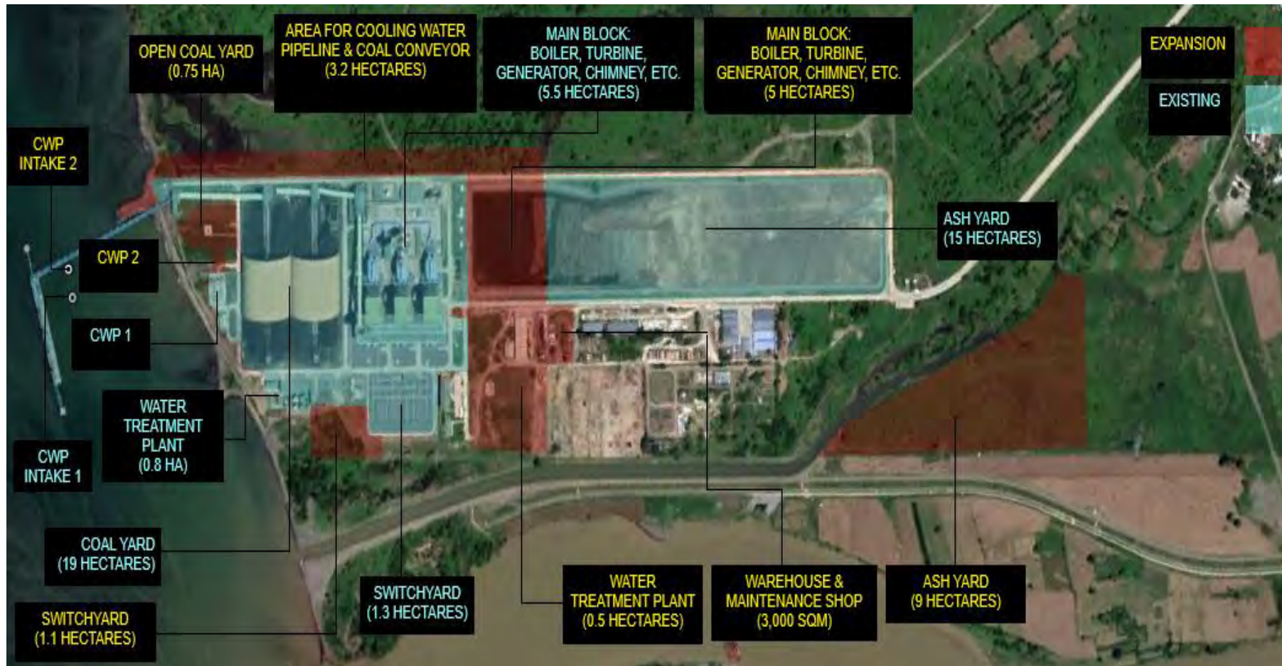
Figure 1-16 Proposed Layout/Footprints of Project Facilities (Existing and Expansion)
