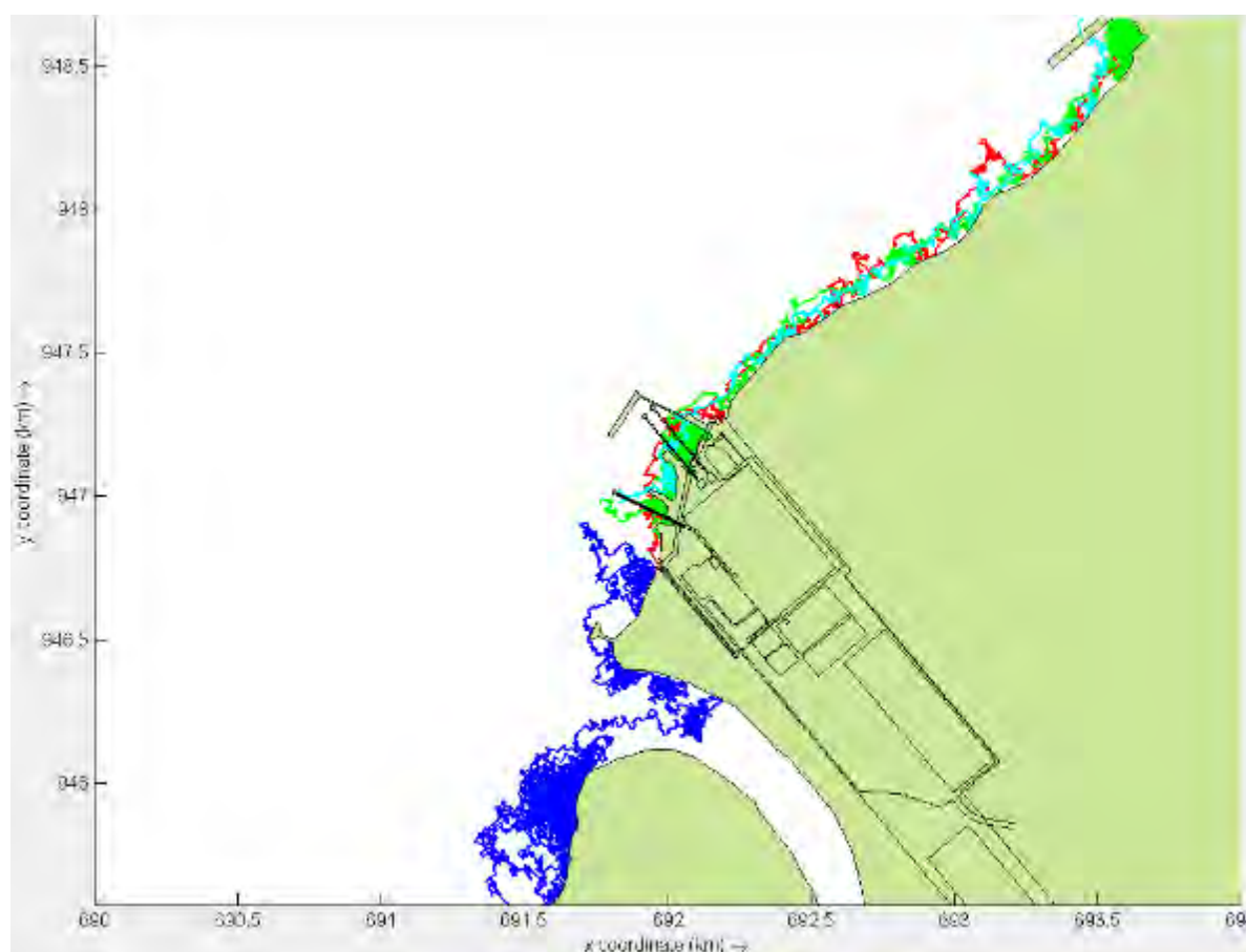
Figure 2.2-36. Predicted trajectories of four (4) particles released at the two outfalls using a Particle Tracking Model
