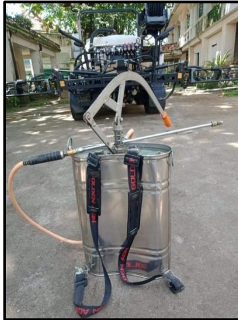
FIGURE 1-16. STAINLESS KNAPSACK SPRAYER ( Tung Ho SA-16 Golden Agin ) USED IN THE APPLICATION OF PESTICIDES
