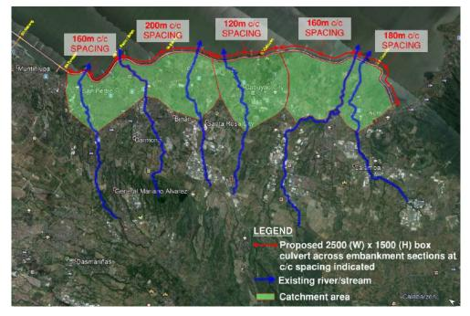
Figure 1-69 Catchment Area Plan of the Overland Flow
