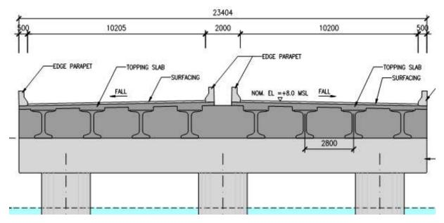
Figure 1-34 Typical Section of Embankment Viaduct with NU Girder
