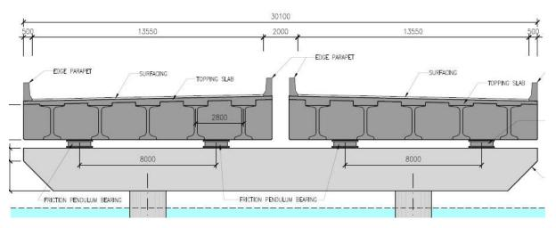
Figure 1-24 Typical Section of Lake Viaduct with AASHTO/NU Girder
