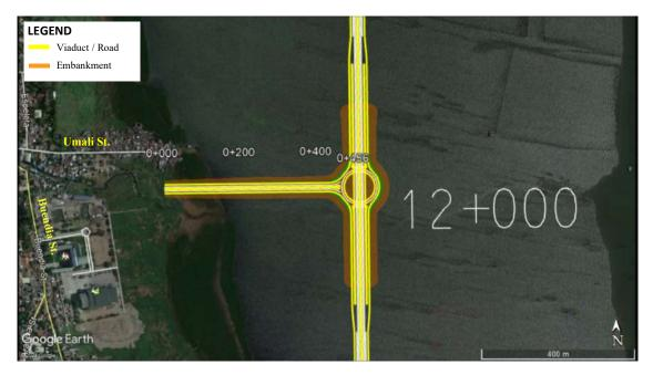
Figure 1-58 Proposed Grade-Separated Roundabout Interchange, Tunasan Interchange
