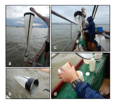
**Plate 3** (a) Operation of 335 microns bongo net with 50 cm mouth diameter and 2.5 meters length for fish eggs and larvae sampling; (b) horizontal tow of the net for 10 minutes; (c) transferring of sample from the bucket to 1-liter capacity plastic bottle; and (d) sieving, storing and preserving of sample with 10% formalin
