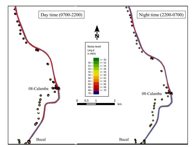
Figure 2.197 Predicted Noise Level (Unmitigated) at NSRs near Calamba & Bucal
