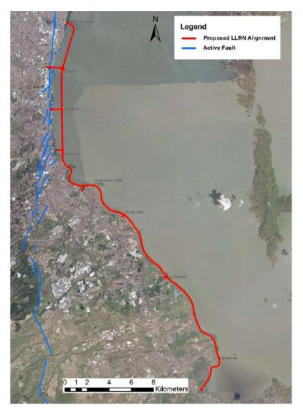
Figure 2-32 Extent of active fault near proposed alignment (PHIVOLCS, 2019)
