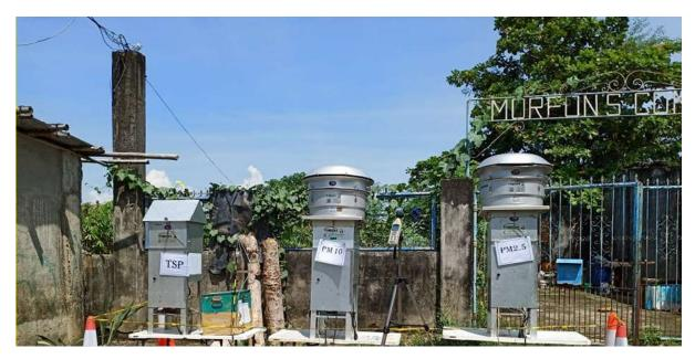
Figure 2.172 Ambient Air Sampling Set-up
