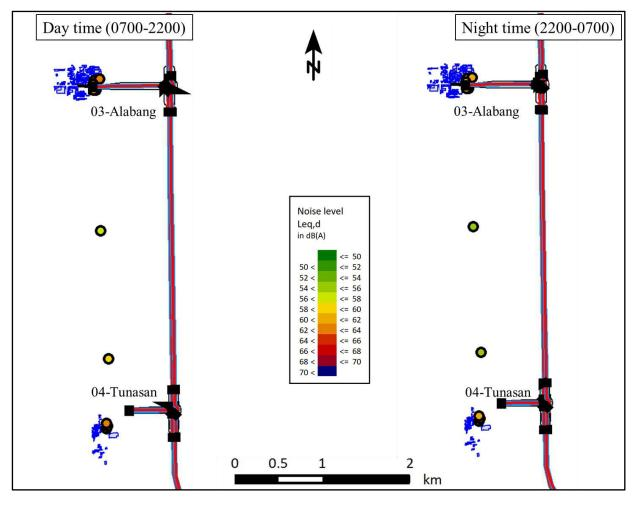
Figure 2.193 Predicted Noise Level (Unmitigated) at NSRs near Alabang & Tunasan
