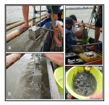
**Plate 4** (a) Lowering of Ekman bottom grab sampler for sediment sampling for soft bottom infaunal benthos, (b) hauling of bottom grab sampler with collected sediment, (c) transferring of sediment sample onto plastic basin, and (d) mud sediment sample obtained for sieving
