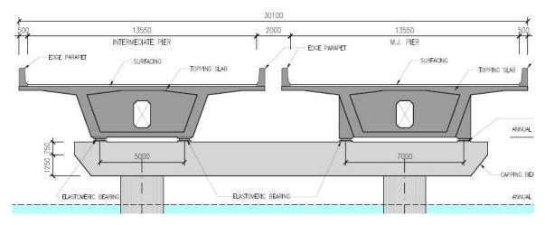
Figure 1-26 Typical Section of Lake Viaduct with Box Girder
