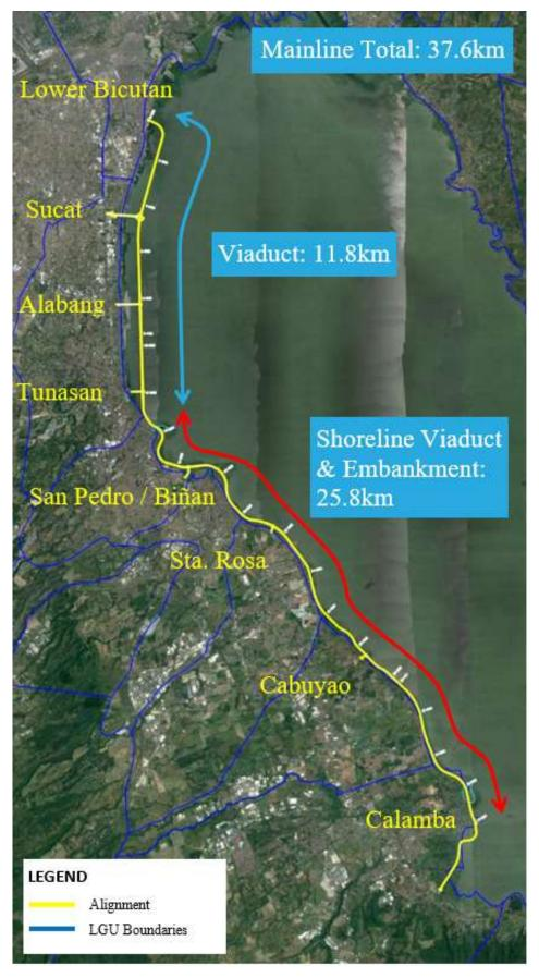
Figure 1-18 LLRN Phase I Final Confirmed Alignment along the Western Coast of Laguna Lake
