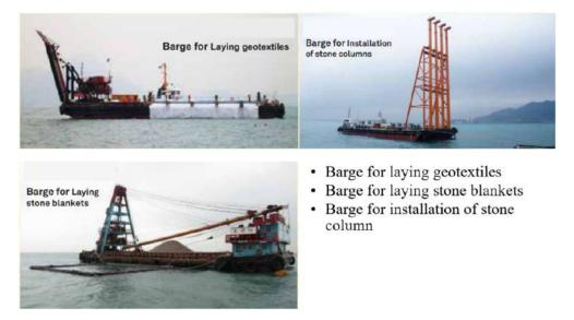
Figure 1-95 Stone Column Installation
