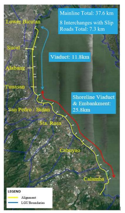
Figure 1-2 LLRN Phase I Final Confirmed Alignment along the Western Coast of Laguna Lake
