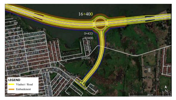
Figure 1-59 Proposed Grade-Separated Roundabout Interchange, San Pedro / Binan Interchange
