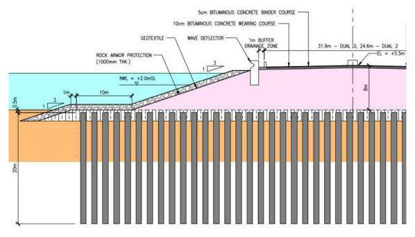
Figure 1-43 Typical Embankment Foundation Detail with Stone Column ground treatment
