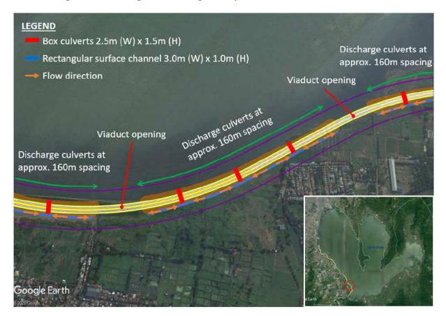
Figure 1-71 Preliminary Drainage Scheme at Shoreline Embankment
