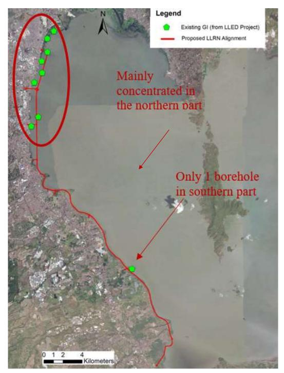
Figure 1-42 Existing Borehole Data Locations Along the Alignment
