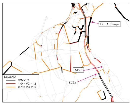
Figure 2-101 Network Performance in V/C ratio for 2035 AM "without project" case
