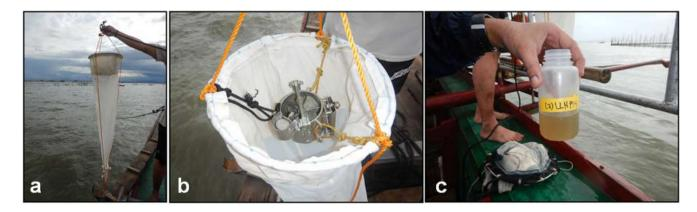
**Plate 1** (a) Phytoplankton sampling by 30 cm mouth diameter, 20  $\mu$ m mesh size and 1 meter length plankton net, (b) flowmeter attached to the center of the mouth of the net, (c) and phytoplankton sample collected
