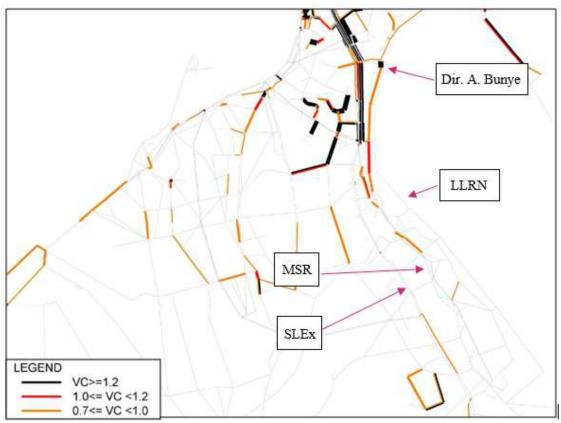
Figure 2-100 Network Performance in V/C ratio for 2025 AM "with project" case
