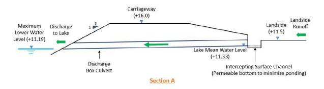
Figure 1-72 Typical Cross-Section of Drainage System at Shoreline Embankment
