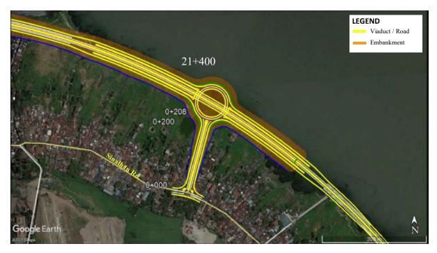
Figure 1-60 Proposed Grade-Separated Roundabout Interchange, Sta. Rosa Interchange
