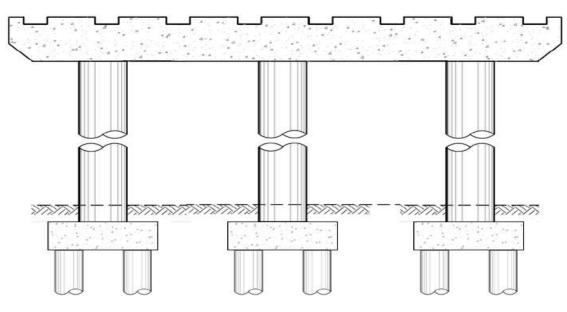
Figure 1-52 Typical Substructure Configuration
