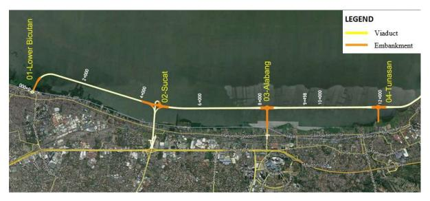
Figure 1-21 Viaduct Section of Mainline Alignment
