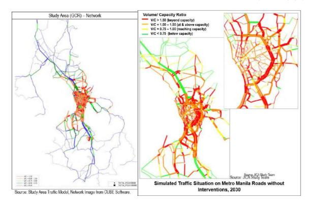
Figure 1-9 Traffic Model- Highway Network Traffic Volume and V/C Ratio<sup>4.5</sup>
