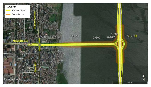
Figure 1-57 Proposed Grade-Separated Roundabout Interchange, Alabang Interchange
