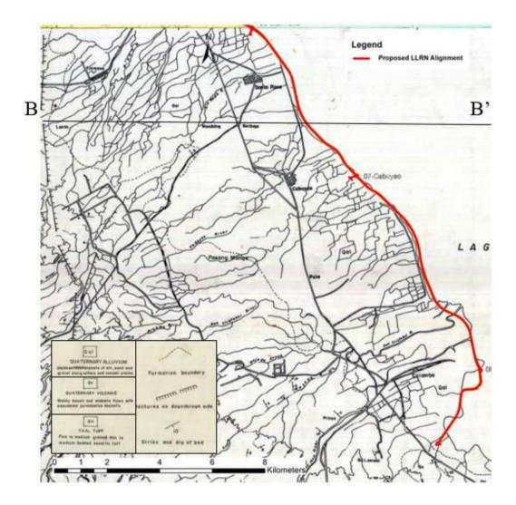
Figure 2-291:50,000-scale Geological map of the project area [Sheet Nos. 3263 III] top and<br/>[Sheet Nos. 3262 IV] bottom (Source: MGB)
