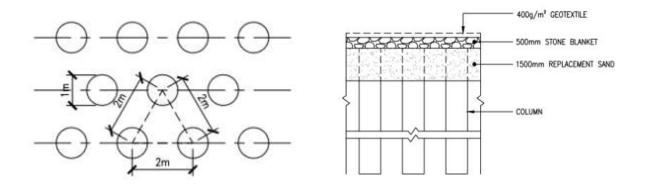
Figure 1-44 Typical Stone Column Layout Plan and Details
