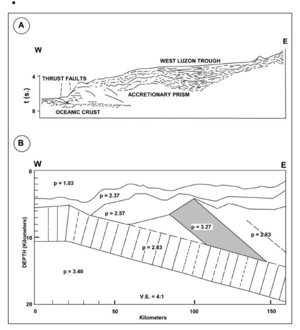
**Figure 2-23** Structure of the accretionary prism of the Manila Trench from seismic profiles (A), and of the subducting slab and over-riding plate established from gravimetric data (B). (MGB, 2010)
