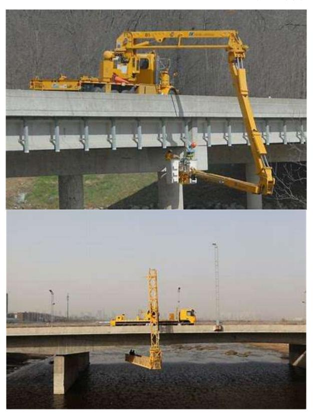
Figure 1-73 Under Bridge Inspection Vehicles (UBIV)
