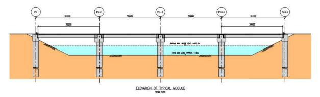
Figure 1-35 Typical Arrangement of Embankment Viaduct
