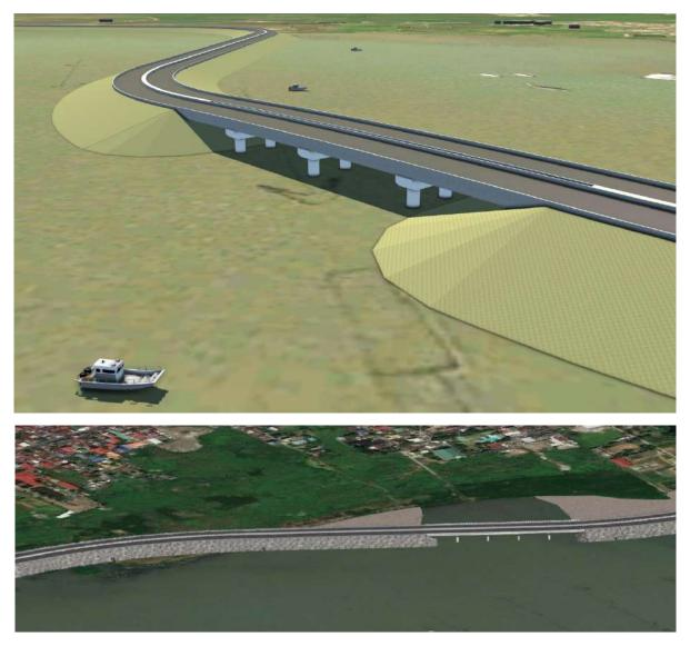
Figure 1-33 Embankment Viaduct at River outlet and fishery basin
