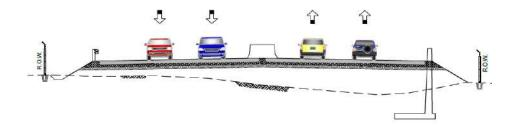
Figure 1-50 Typical Cross Section for Embankment Section
