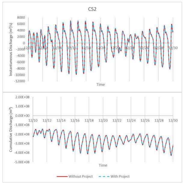
Figure 2.98 Instantaneous Discharge and Cumulative Discharge at "CS2"
