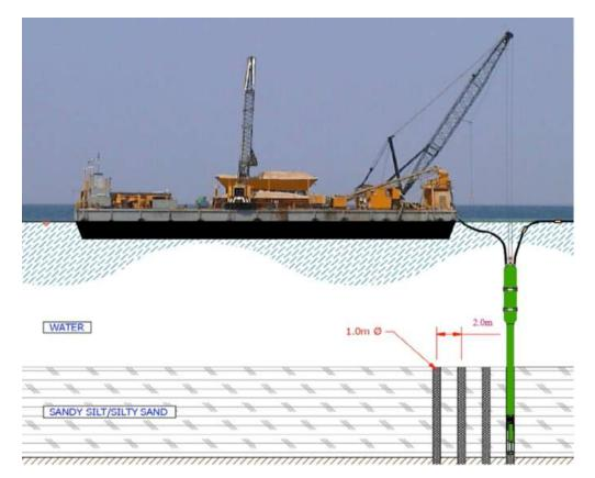
Figure 1-94 Stone Column Construction
