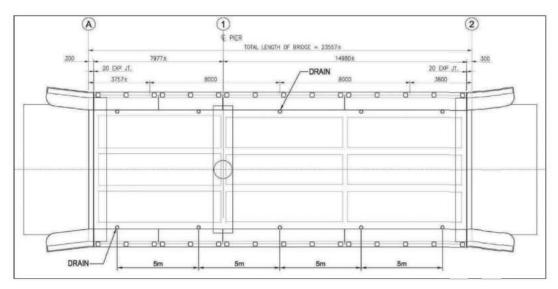
Figure 1-66 Spacing of Bridge Drains
