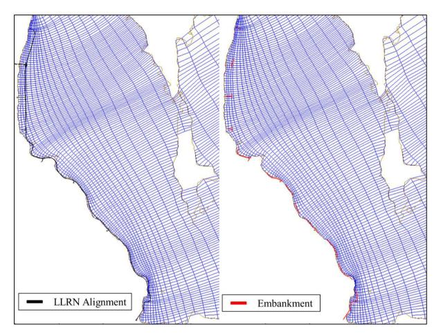
Figure 2.93 LLRN Alignment, Embankment and Model Grid
