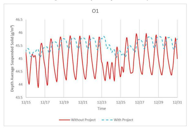
Figure 2.106 Depth Average Suspended Solids at "O1"
