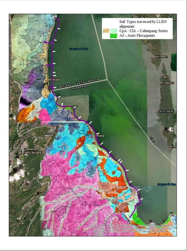
Figure 2-46 Published Soil Type Map along the LLRN - PH1Alignment adapted from BSWM
