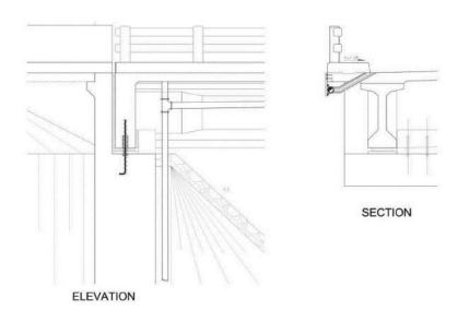
Figure 1-68 Lateral Pipe Ending to a Downspout
