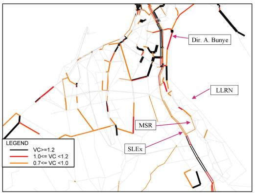
Figure 2-102 Network Performance in V/C ratio for 2035 AM "with project" case
