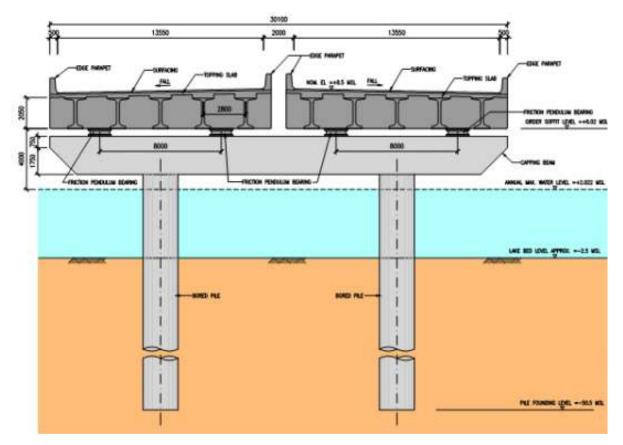
Figure 1-32 In-lake viaduct cross section and arrangement
