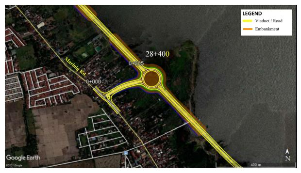
Figure 1-61 Proposed Roundabout Interchange Option, Cabuyao Interchange
