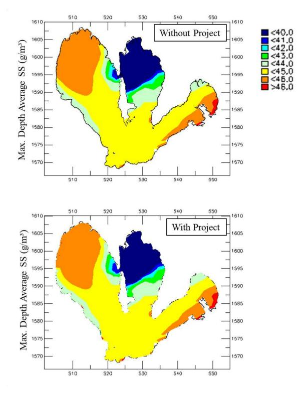
Figure 2.101 Contour Plot for Max. Depth Average Suspended Solid
