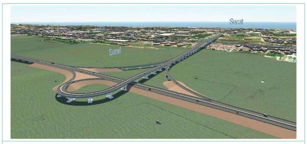
Trumpet interchange is a 3-leg interchange which takes the shape of trumpet. Trumpet interchanges have been used where one connection terminates at the highway mainline. This layout involves loop ramps connecting traffic entering or leaving the mainline with the far side of continuous highway. This type of interchange allows for free flow of traffic in all direction.
