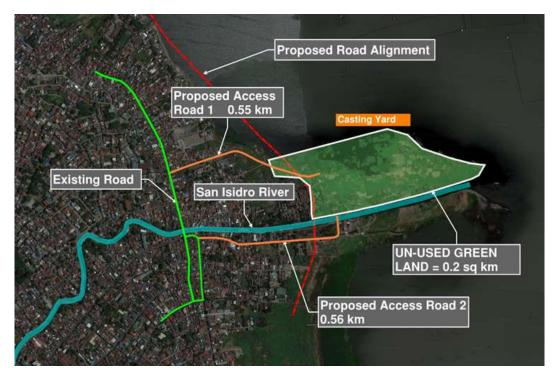
Figure 1-76 Possible Location of Casting Yard 1
