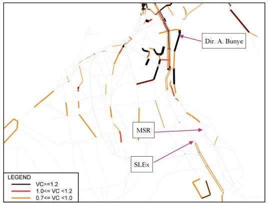
Figure 2-99 Network Performance in V/C ratio for 2025 AM "without project" case
