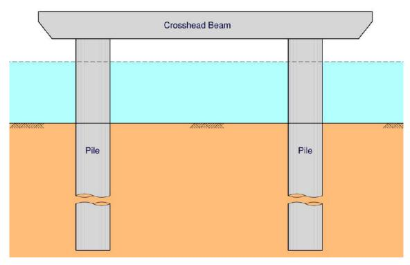
Figure 1-31 Typical Arrangement of Crosshead Beam
