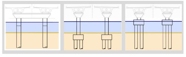
Figure 1-28 Monopile without Pile Cap
